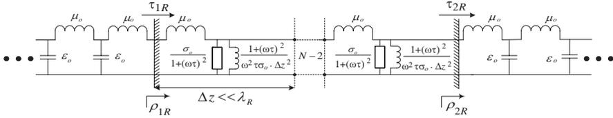
**Figure 6.** Equivalent transmission line model for predicting metal shielding behaviour, using the classical relaxation-effect model and showing expressions for the distributed-element parameters (e.g.,  $L_R \cdot \Delta z = 1.341$  [fH],  $G_R \cdot \Delta z = 24.1$  [mS] and  $L_{SHUNT,R} \cdot \Delta z = 1.126$  [pH] at 5.865 THz for gold at room temperature [5, 6]).
