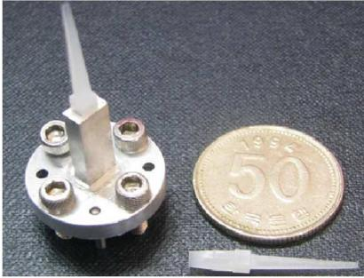
**Figure 3.** Dielectric rod waveguide antenna.
