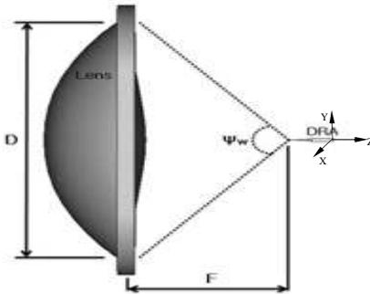
**Figure 6.** Quasi-optics configuration of the lens and DRW.
