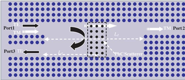
**Figure 1.** The schematic configuration of the proposed PBS.
