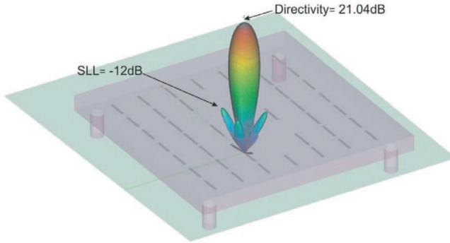
**Figure 10.** Geometry and power pattern radiated by a design of 49 parasitic elements placed  $0.59\lambda$  in front of a finite ground plane and taking into account the dielectric substrate and the teflon screws.
