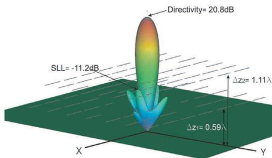
**Figure 9.** Geometry and power pattern radiated by the antenna of two layers composed by 49 parasitic elements placed  $0.59\lambda$  and  $1.11\lambda$  in front of a finite ground plane and with a pure real active impedance of  $75 \Omega$ .
