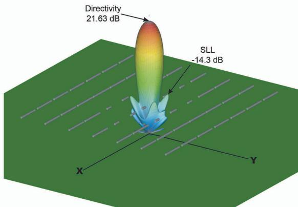
**Figure 2.** Geometry and power pattern radiated by the antenna of 49 parasitic elements placed  $0.59\lambda$  in front of an infinite ground plane.
