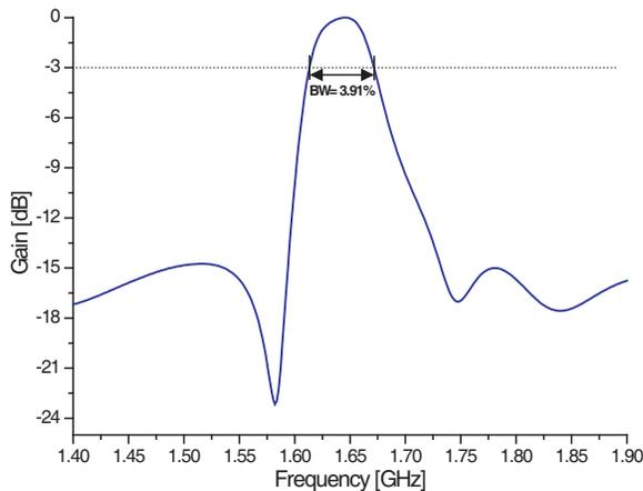
**Figure 5.** Antenna gain versus frequency for the antenna of Fig. 4.
