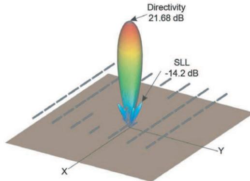
**Figure 4.** Geometry and power pattern radiated by the antenna of Fig. 2 after applying array thinning. A more realistic simulation has been performed by considering a finite ground plane and the electromagnetic characteristics of the copper.
