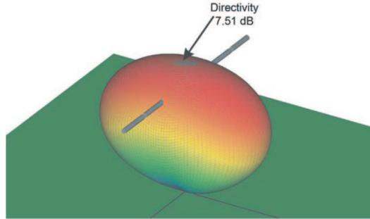
**Figure 3.** Power pattern radiated by a  $\lambda/2$ -dipole placed  $\lambda/4$  in front of a ground plane.
