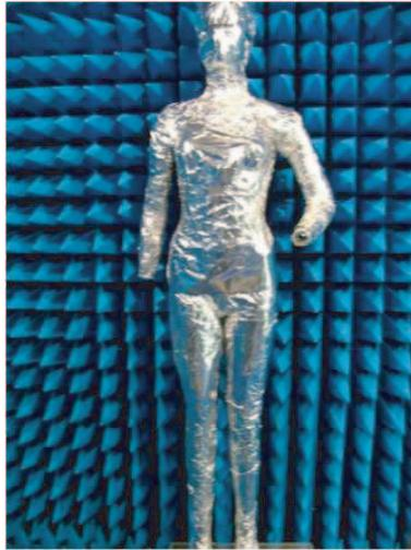
**Figure 3.** Picture of the mannequin within the anechoic chamber.
