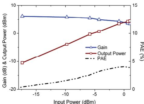
**Figure 16.** Measured output power and gain VS input power at 135 GHz.
