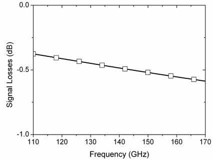
**Figure 6.** RF signal loss of 100- $\mu\text{m}$  thin-film microstrip line.
