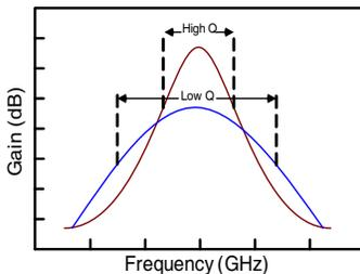
Figure 12. Impact of  $Q$  on bandwidth.
