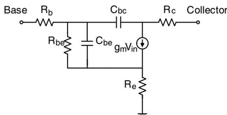
**Figure 1.** Small signal model of SiGe HBT transistor.
