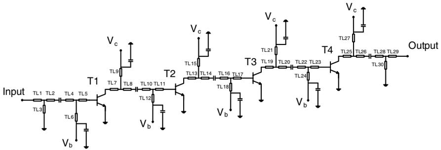
**Figure 4.** Schematic of proposed 4-stage common-emitter power amplifier.
