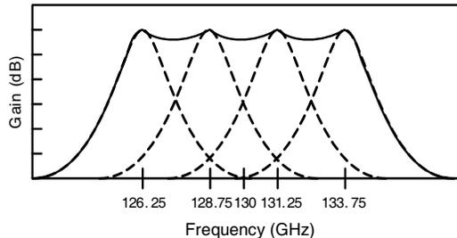
Figure 13. Frequency response of wideband power amplifier.
