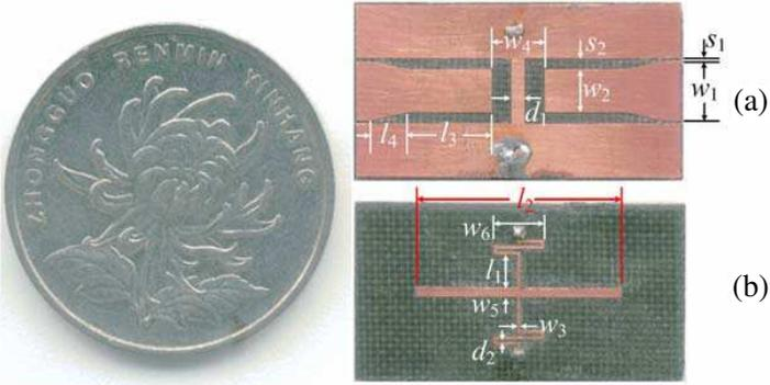
**Figure 4.** Photograph of the fabricated UWB BPF: (a) top view and (b) bottom view. ( $s_1 = 0.22$  mm,  $s_2 = 0.87$  mm,  $w_1 = 4.5$  mm,  $w_2 = 3.2$  mm,  $w_3 = 0.22$  mm,  $w_4 = 4$  mm,  $w_5 = 0.7$  mm,  $w_6 = 4$  mm,  $l_1 = 2.5$  mm,  $l_2 = 15$  mm,  $l_3 = 6.25$  mm,  $l_4 = 3$  mm,  $d_1 = 1$  mm and  $d_2 = 0.22$  mm)
