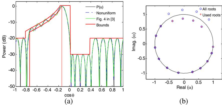
**Figure 3.** Synthesis of a nonsymmetrical pattern: (a) the pattern  $P(u)$ , the pattern reconstructed by 13 nonuniformly spaced elements, and the pattern synthesized by [3]; (b) distribution of the roots of the polynomial associated with the power pattern.
