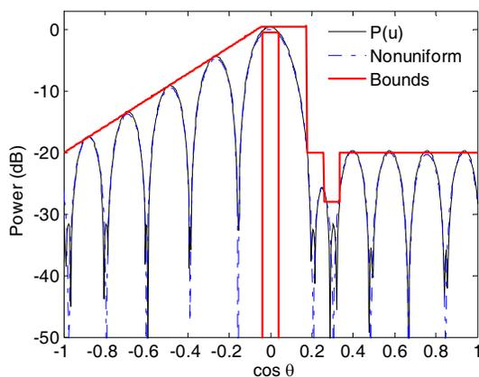
**Figure 5.** Pattern synthesis of the transmitting antenna array.
