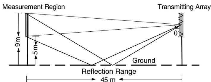
**Figure 4.** Geometry of an outdoor antenna test range.
