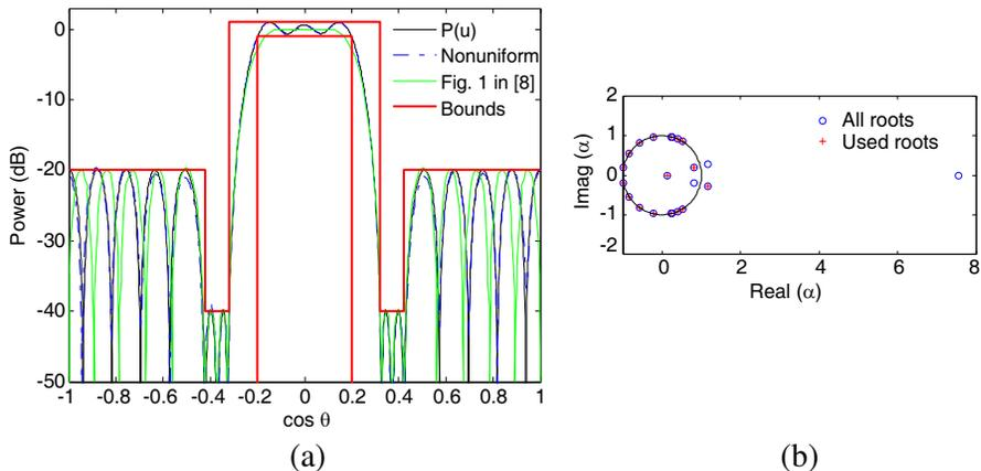
**Figure 2.** Synthesis of a flap-top pattern: (a) the pattern  $P(u)$ , the pattern reconstructed by 12 nonuniformly spaced elements, and the pattern synthesized by [8]; (b) distribution of the roots of the polynomial associated with the power pattern.
