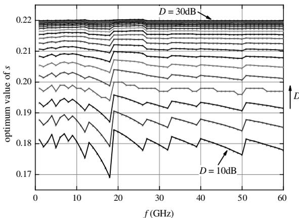
**Figure 3.** Optimal values for  $s$  versus frequency at  $D = 10, 11, \dots, 30$  dB.
