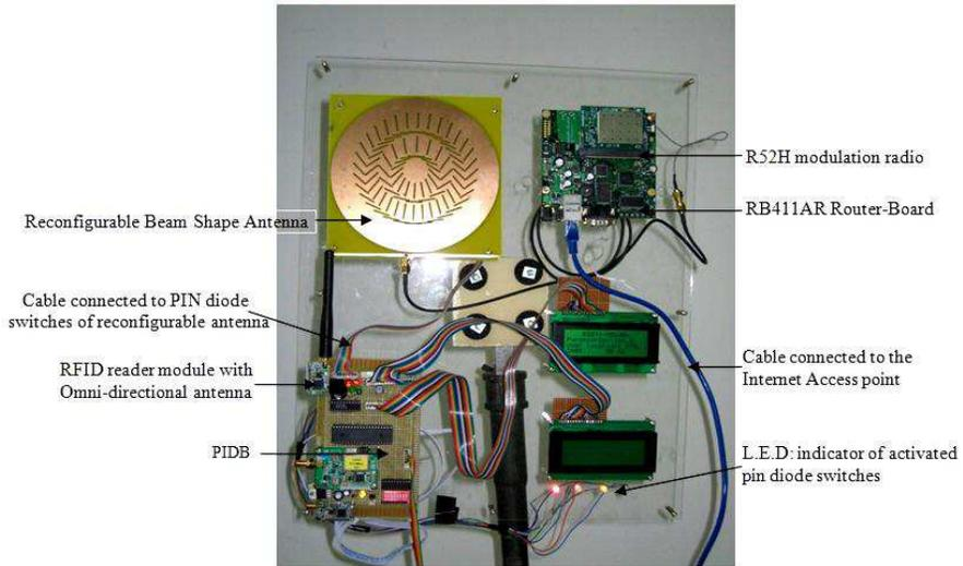
**Figure 5.** Complete prototype of adaptive Wi-Fi system.
