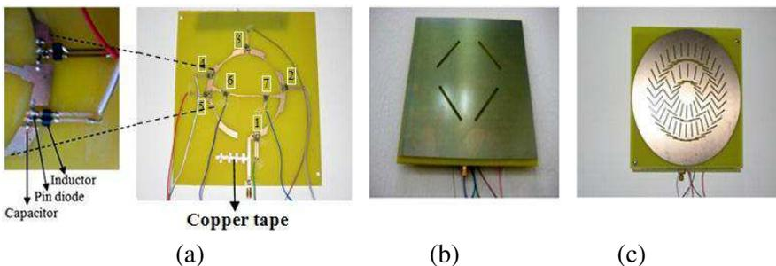
**Figure 2.** The reconfigurable beam shaped antenna [1], (a) feed line with PIN diode switches, (b) aperture slots, (c) RLSA radiating surface.
