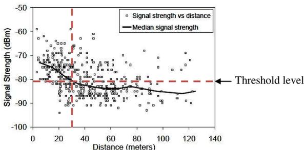
Figure 1. Wi-Fi signal strength over distance [14].
