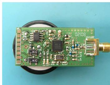
**Figure 5.** SMA connectorized antenna implementation of GMSK transmitter.
