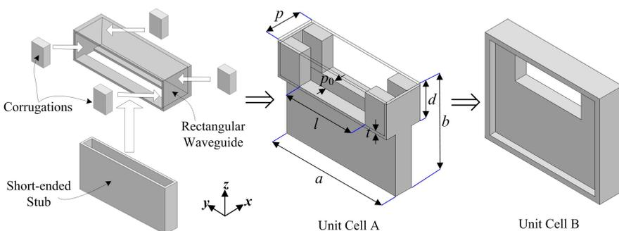
**Figure 3.** Another equivalent form of the proposed CRLH waveguide unit cell. It is composed of a section of rectangular waveguide, corrugations on both sidewalls and a short-ended stub on the bottom wall of the rectangular waveguide. Some place is set to be transparent for convenient viewing. The parameters are the same with that in Fig. 2.
