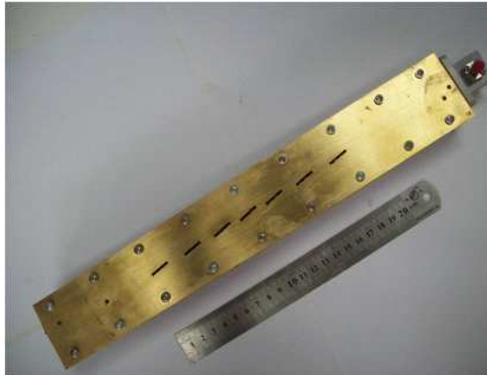
**Figure 10.** Prototype of a seven-element unequally spaced and excited resonant slotted-waveguide antenna array.
