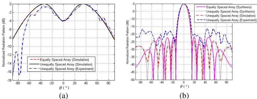
**Figure 11.** Comparison of far-field radiation patterns between the equally spaced and unequally spaced arrays. (Freq = 10 GHz). (a) *H*-plane (*y*-*z* plane,  $\phi = 90^\circ$ ) (b) *E*-plane (*x*-*z* plane,  $\phi = 0^\circ$ ).
