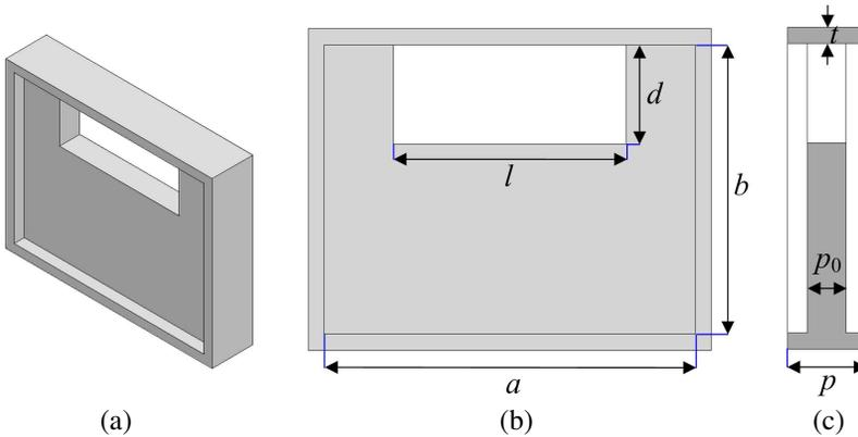
**Figure 2.** Structure of the improved CRLH waveguide unit cell. ( $a = 23.4$  mm,  $b = 18.1$  mm,  $l = 14.65$  mm,  $d = 6.2$  mm,  $p = 5$  mm,  $p_0 = 2.5$  mm and  $t = 1$  mm). (a) General view. (b) Front view. (c) Side view.
