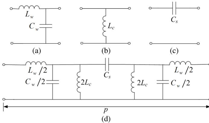
**Figure 4.** Equivalent circuit model of the unit cell and its component parts. (a) Equivalent circuit of rectangular waveguide. (b) Equivalent circuit of corrugations. (c) Equivalent circuit of short-ended stub. (d) Equivalent circuit model of unit cell.
