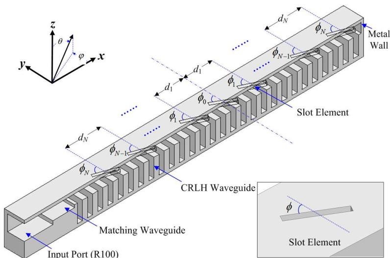
**Figure 1.** Longitudinal section of an unequally spaced and excited resonant slotted-waveguide antenna array employing the proposed CRLH waveguide. Centered rotated slots, symmetrically situated and excited, are used here, and one of them is shown in the inset. The antenna array is excited by an end-fed structure.  $d_i$  and  $\phi_i$  ( $i = 1, 2, \dots, N$ ) represent the  $i$ th adjacent element spacing, and the  $i$ th slot rotation angle with respect to the  $y$ -axis, respectively.
