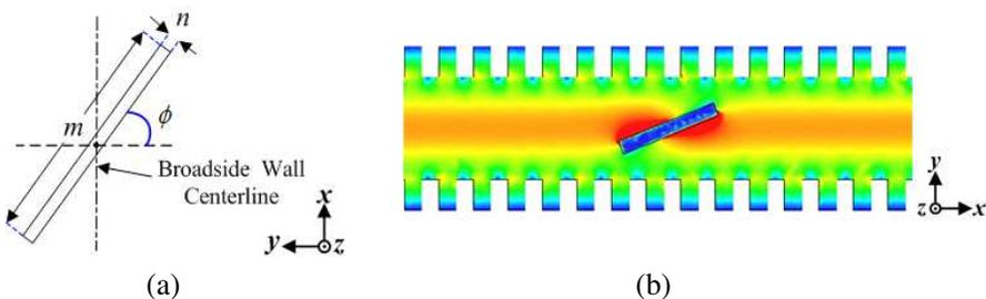
**Figure 8.** Slot used in this paper and its radiation mechanism. (a) Geometry and parameters of the slot ( $m = 14.8$  mm and  $n = 2$  mm). (b) Surface current interruption by the slot.
