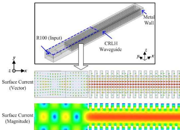
**Figure 7.** Illustration of a standing wave in the shorted CRLH waveguides with the mapping of the surface current. The CRLH waveguides are excited by an end-fed structure with R100 waveguide as an input port.
