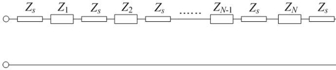
**Figure 9.** Transmission line circuit model of the proposed antenna array.  $Z_i$  ( $i = 1, 2, \dots, N$ ) and  $Z_s$  represent the  $i$ th series impedances of the slot and the characteristic impedance of CRLH waveguide, respectively.
