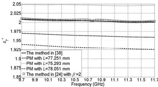
**Figure 2.** Measured real part of  $\epsilon_r$  of the PTFE sample ( $L = 76.28$  mm) using our proposed method and the methods in [24] and [38]. In the figure, PM refers to the abbreviation of the proposed method.
