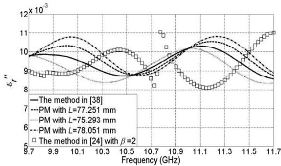
**Figure 3.** Measured imaginary part of  $\epsilon_r$  of the PTFE sample ( $L = 76.28$  mm) using our proposed method and the methods in [24] and [38]. In the figure, PM refers to the abbreviation of the proposed method.
