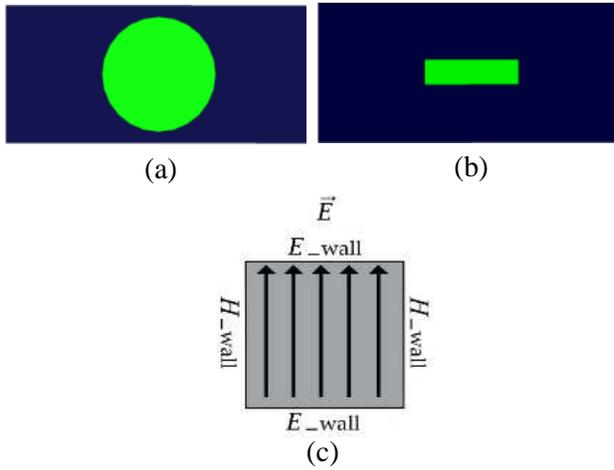
**Figure 2.** Array element: (a) Top view, (b) bottom view and (c) equivalent unit cell waveguide model.
