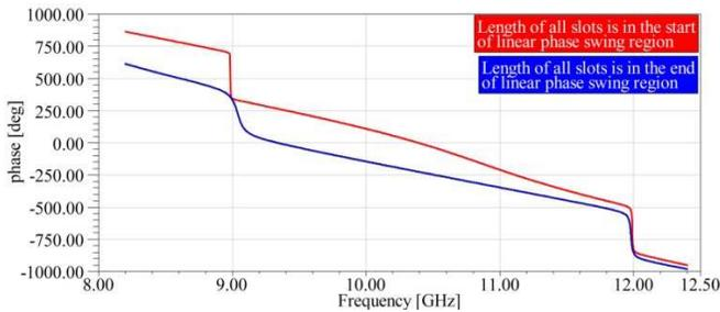
**Figure 7.** Bandwidth of reflectarray using circular patch elements.
