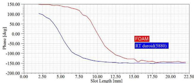
Figure 4. Reflection phase for various substrate permittivity.
