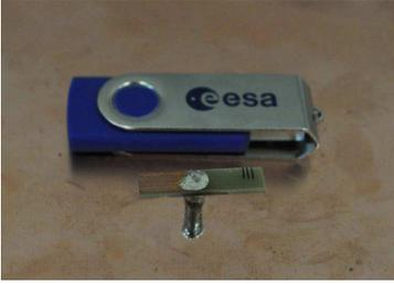
**Figure 4.** Photograph of the feeder fixed and soldered above the ground plane.
