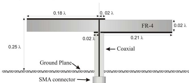
**Figure 3.** Dipole geometry.
