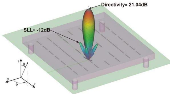
**Figure 2.** Power pattern simulated by the antenna composed of 41 parasitic elements placed  $0.59\lambda$  in front of a finite ground plane; the dielectric substrate and the Teflon screws have been taken into account.
