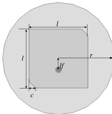
Figure 5. Geometry of the circularly-polarized microstrip patch antenna.
