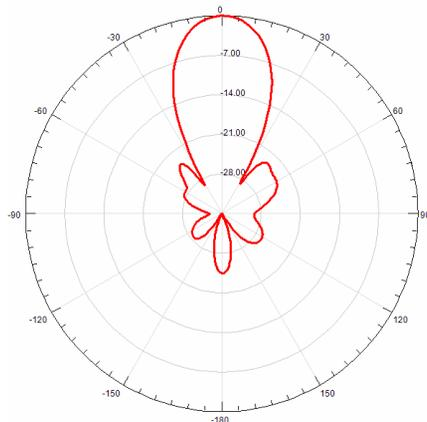
**Figure 8.** Synthesized radiation pattern for low sidelobe.
