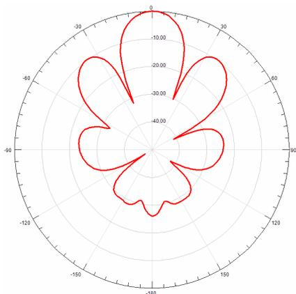
**Figure 7.** Radiation patterns of the array before synthesis.
