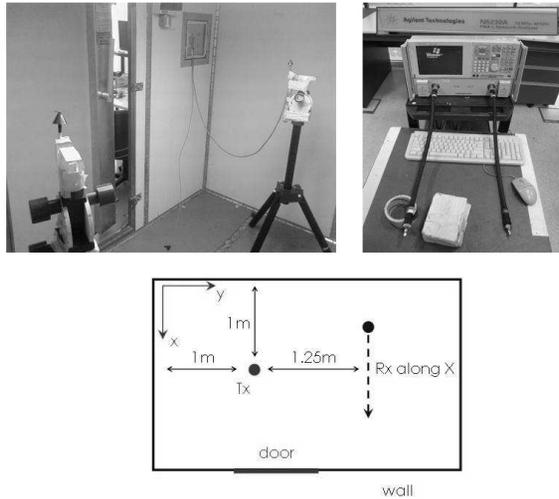
**Figure 6.** Measurements conducted for the signal propagation between two disc-cones inside a shielding room by using a Vector Network Analyzer (HP 8753E), which generates the transmitted power ( $P_t = -10$  dBm) and captures the signal at the receiver over the entire measurement frequency (2.8 GHz to 3.2 GHz). The 2D cut-plane shows the locations of the Tx and Rx according to the origin of the coordinate system. Tx and Rx are above the floor at the same height of 1 m.
