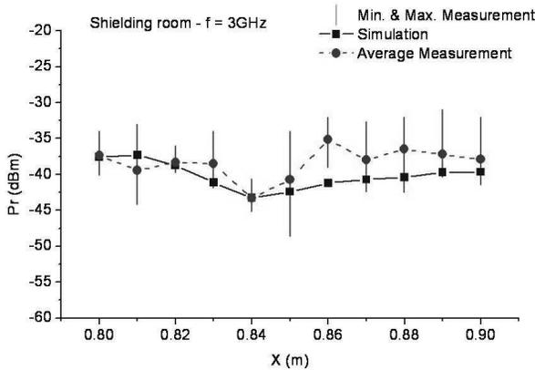
**Figure 7.** Comparison between the simulated results and the measurements (averaged value/range of the minimum and maximum values) — Received power in dBm recorded along  $X$  direction.
