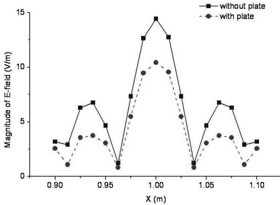
**Figure 5.** Comparison between the models with and without plate — Magnitude of the electric field along  $X$  direction at  $(x_r, y_r, z_r) = (X, 2.25, 1.0)$ . Transmitting antenna is located at coordinates  $(x_t, y_t, z_t) = (0.97, 1, 1)$ . All dimensions are in meter.
