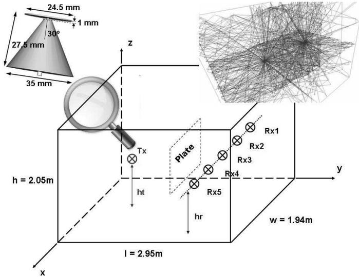
**Figure 4.** An enclosed room made by metal wall ( $\sigma = 11000 \text{ S/m}$ ) with dimensions of 1.94 width, 2.95 length, and 2.05 height. A metal plate with dimensions of  $0.94 \times 1$  placed at  $(x_{pmin} - x_{pmax}, y_p, z_{pmin} - z_{pmax}) = (0.5 - 1.44, 1.75, 0.5 - 1.5)$  used as furniture placed inside this room to block the Line-Of-Sight (LOS) between transmitting antenna and the receiving points. All dimensions are in meter.
