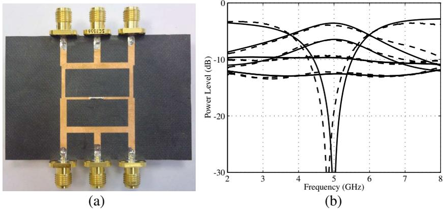
**Figure 7.** Power divider with 1:4:2:8 power ratio. (a) A photograph of the fabricated structure. (b) Simulation (ADS Momentum) and measurement results. Dashed lines are measured and solid lines are simulated power levels.
