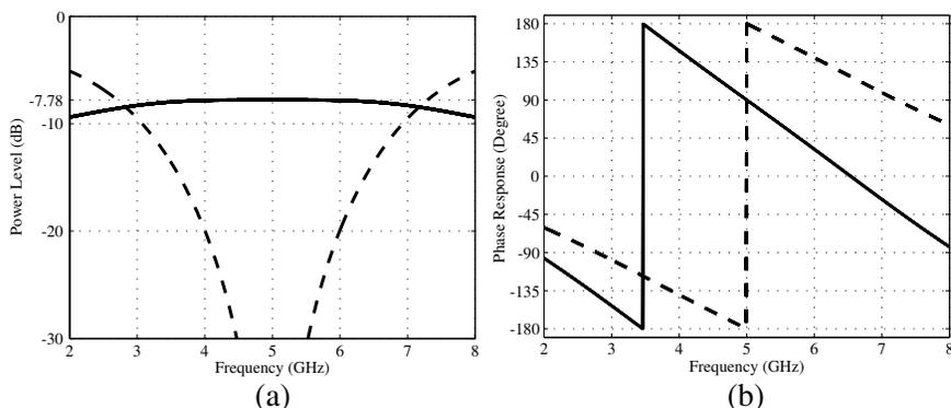
**Figure 2.** Simulation results for an ideal power divider with 1:1:1:1 power ratio. (a) Solid curve is the output power level in dB relative to input power at the 6 output ports ( $P = -7.78$  dB) and dashed curve is the reflection coefficient  $|S_{77}|^2$ . (b) Solid line is the phase responses of  $S_{27}$  and  $S_{57}$ . Dashed line is the phase response at ports  $S_{17}$ ,  $S_{37}$ ,  $S_{47}$ , and  $S_{67}$ .
