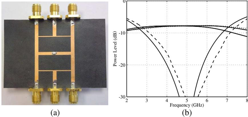
**Figure 5.** Power divider with 1:1:1:1 power ratio. (a) A photograph of the fabricated structure. (b) Simulation (ADS Momentum) and measurement results. Dashed lines are measured and solid lines are simulated power levels.
