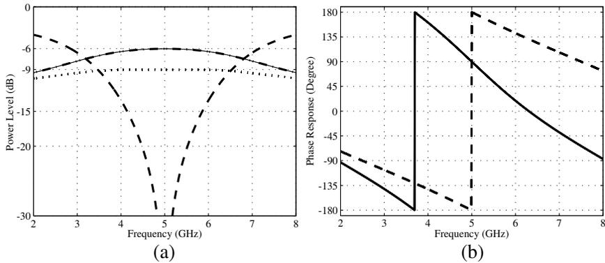
**Figure 3.** Simulation results for an ideal power divider with 1:2:1:2 power ratios in dB relative to input power. (a) Solid curve is the output power level at  $P_2$  and  $P_5 = -6$  dB. Dotted curve is the output power level at  $P_1$  and  $P_4 = -9$  dB. Dashed curve is the reflection coefficient  $|S_{77}|^2$ . (b) Solid line is the phase response of  $S_{27}$  and  $S_{57}$ , and dashed line is the phase response at ports  $S_{17}$ ,  $S_{37}$ ,  $S_{47}$ , and  $S_{67}$ .
