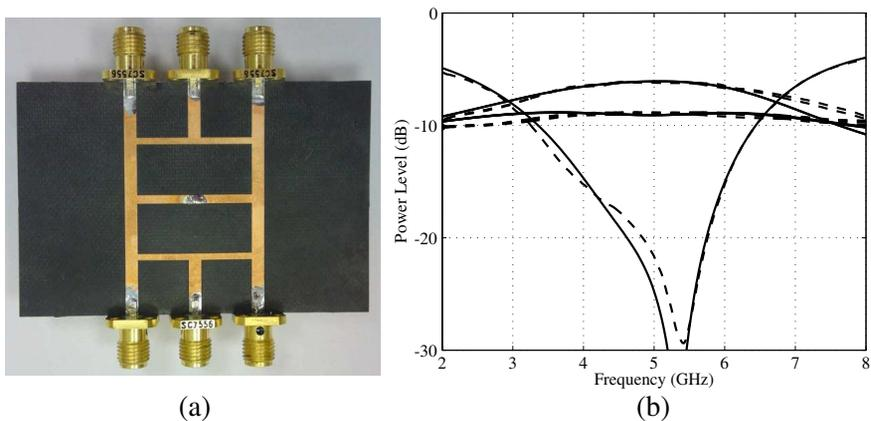
**Figure 6.** Power divider with 1:2:1:2 power ratio. (a) A photograph of the fabricated structure. (b) Simulation (ADS Momentum) and measurement results. Dashed lines are measured and solid lines are simulated power levels.
