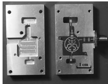
**Figure 10.** Photo of the single balanced mixer.
