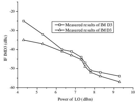
**Figure 14.** IF IMD3 vs. LO power with -15 dBm RF power at 30.2 GHz.
