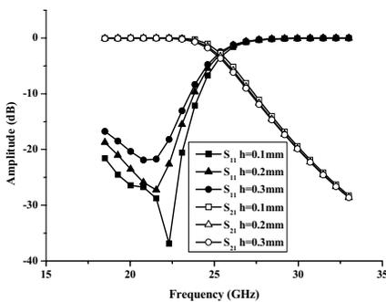
**Figure 9.** Simulated results of the lowpass filter.
