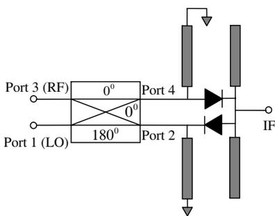
**Figure 3.** Schematic of the single balanced mixer.
