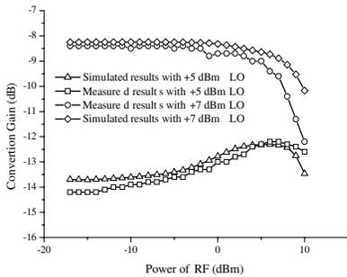
**Figure 13.** Power of RF vs. conversion gain at +5 and +7 dBm drive level at 30.2 GHz RF frequency.
