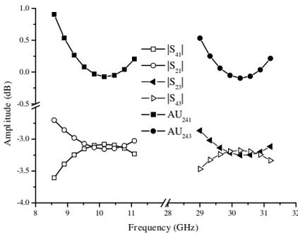
**Figure 5.** Amplitude unbalance of the rat-race ring.
