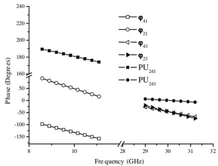
**Figure 6.** Phase unbalance of the rat-race ring.
