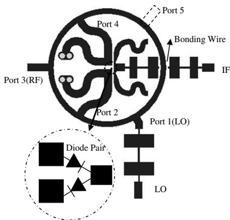
**Figure 4.** Layout of the single balanced mixer.
