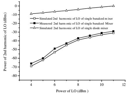
**Figure 12.** Power of second harmonic of LO measured at the IF port.
