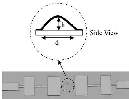
**Figure 8.** Model of the lowpass filter with bonding wires.
