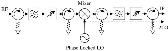
**Figure 1.** Typical diagram of the transponder simulator.
