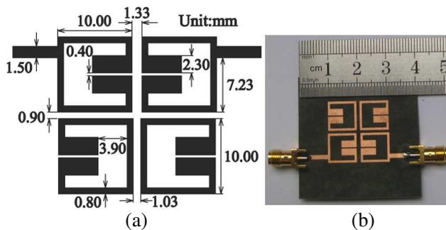
**Figure 6.** (a) Physical dimensions and (b) photograph of the fabricated filter 2.
