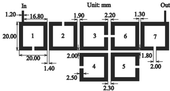
**Figure 3.** Physical dimensions of filter 1.
