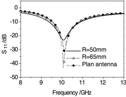
**Figure 2.** Return loss with different curvature radius.
