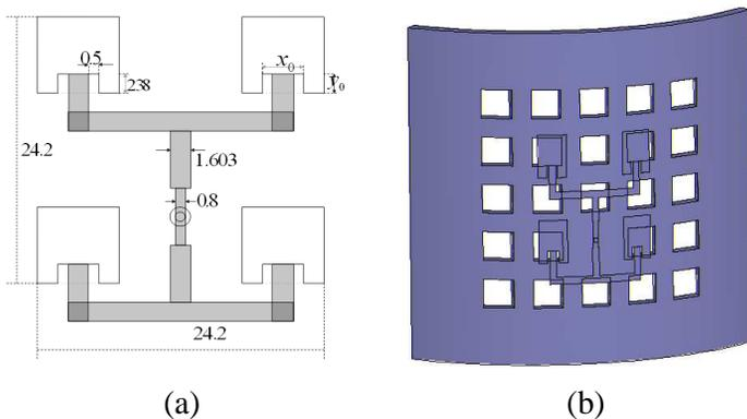
**Figure 9.** Prototype of cylindrical array with PBG lattice: (a) The patch array, (b) the cylindrical structure.
