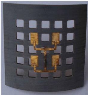
**Figure 10.** Fabricated cylindrical conformal array antenna with PBG lattice.
