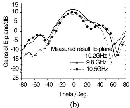
**Figure 12.** Measured radiation pattern of cylindrical array antenna with PBG lattice at different frequencies: (a) *H*-plane, (b) *E*-plane.
