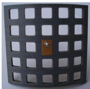
**Figure 6.** Fabricated cylindrical microstrip antenna with PBG lattice.
