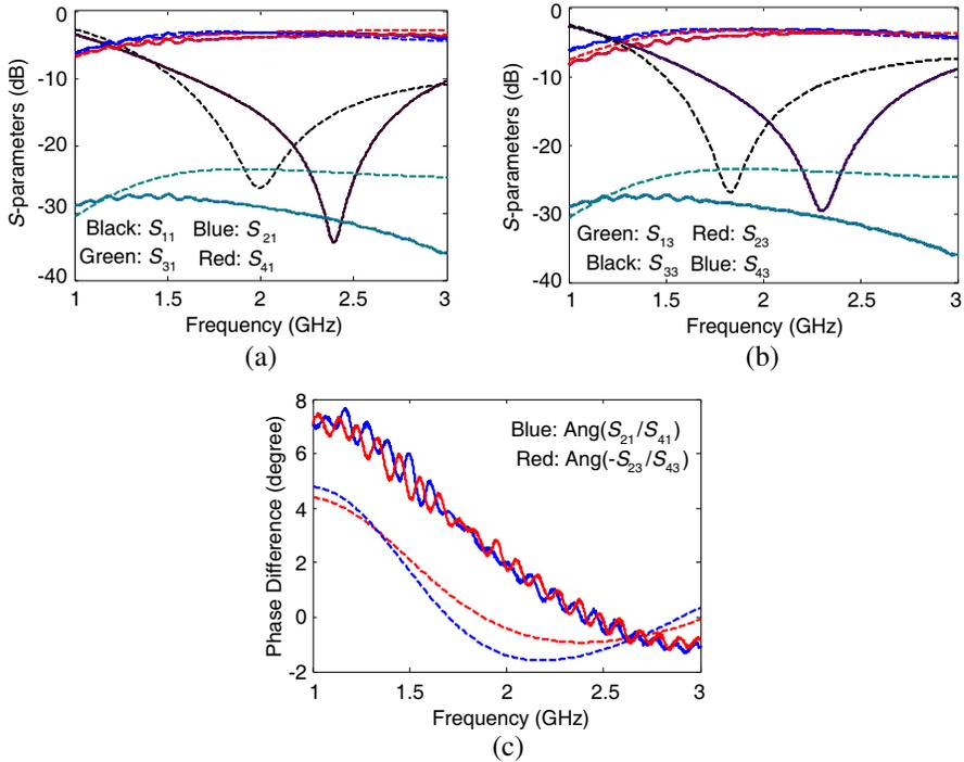
**Figure 10.** Measured and simulated frequency responses of the rat-race coupler prototype, where solid and dashed lines represent measured and simulated results, respectively. (a) In-phase and (b) out-of-phase magnitude responses. (c) Phase differences.
