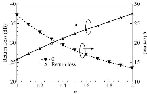
**Figure 2.** The required electric lengths of CPW lines and the associated return losses the proposed baluns that consist of  $\lambda/8$  3 dB couplers and various characteristic impedances of CPW lines.
