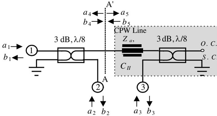
**Figure 1.** Schematic of the proposed miniature balun with incident and reflected wave variables.
