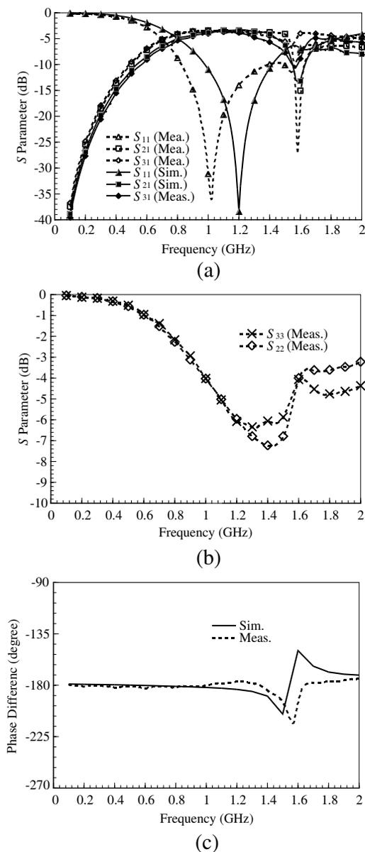
**Figure 7.** Simulated and measured  $S$ -parameters of the balun shown in Fig. 6. (a)  $S_{11}$ ,  $S_{21}$  and  $S_{31}$ , and (b)  $S_{22}$  and  $S_{33}$ . (c) Phase difference between  $S_{21}$  and  $S_{31}$ .
