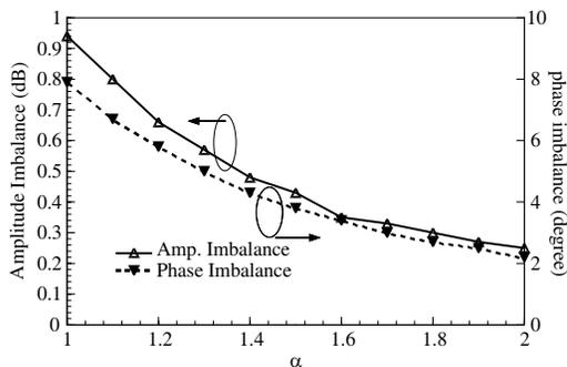
**Figure 3.** The amplitude and phase balances of the proposed baluns constructed with  $\lambda/8$  3 dB couplers and various characteristic impedances of CPW lines having the electric length obtained from Eq. (13).
