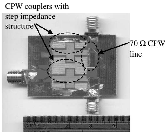
**Figure 6.** Photograph of the CPW balun constructed by length-reduced couplers on FR4 PCB.
