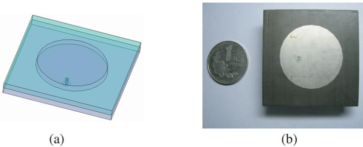
**Figure 2.** (a) Geometry of the coaxial-fed, stacked patch antenna, and (b) photograph of the fabricated antenna.
