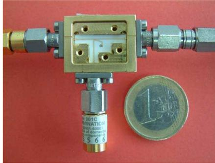
**Figure 8.** View of the designed directional coupler without dielectric overlay for visibility reasons.
