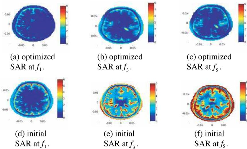
**Figure 8.** Quality indicators parameters for dielectric head-model: SAR.
