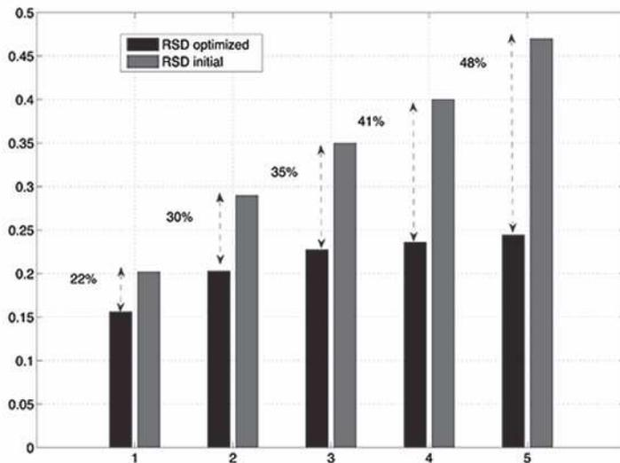
**Figure 12.** Relative standard deviation for all Larmor frequencies: black bar is the RSD for the initial field, light grey bar is the obtained RSD after COPAS. The percentage is related to the relative variation with respect to the initial RSD.
