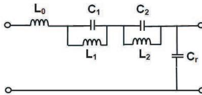
**Figure 4.** The proposed LC-loaded circuit with multiple resonances to support dual-frequency operation.
