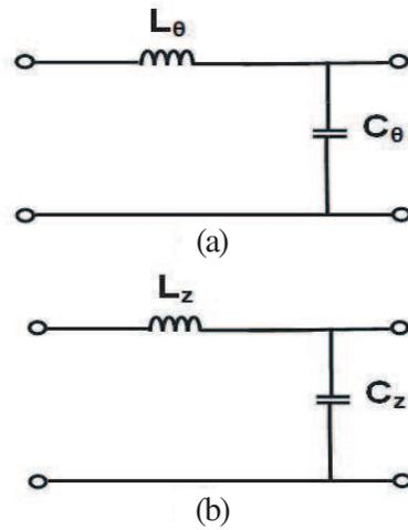
**Figure 3.** Schematics of the LC-loaded circuits for the medium in (a)  $\theta$ -direction and (b)  $z$ -direction.
