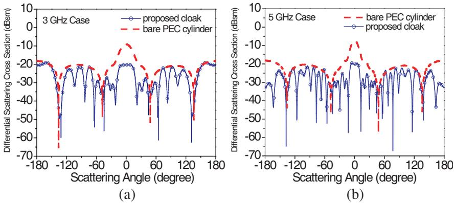
**Figure 6.** The calculated differential scattering cross sections of the proposed cloak along with the results for the bare PEC, (a) at 3 GHz and (b) at 5 GHz.
