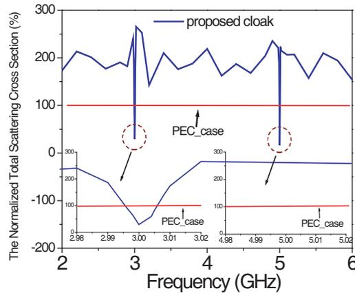
**Figure 7.** Calculated normalized total scattering cross section of the proposed dual-frequency cloak over the frequency range from 2 GHz to 6 GHz.
