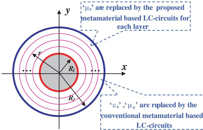
**Figure 1.** Schematic of the proposed dual-band cloak.
