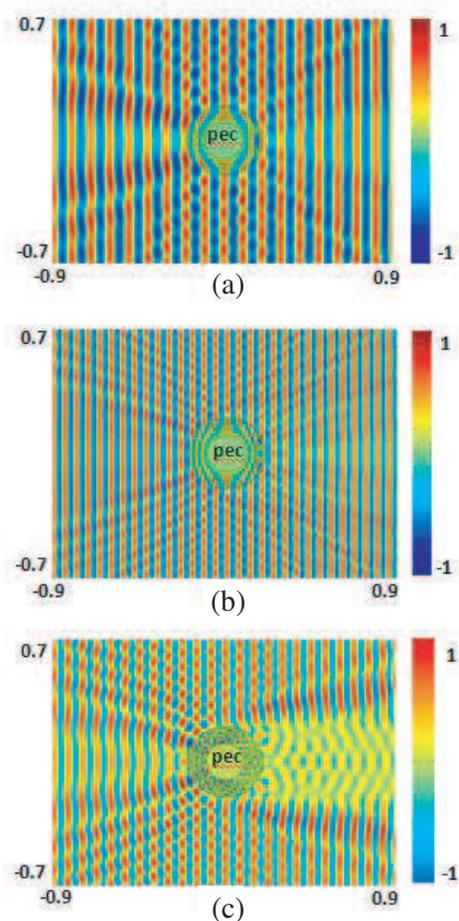
**Figure 5.** The  $E$ -field distributions of the proposed dual-frequency cloak at different frequencies (a) 3 GHz (first working frequency,  $f_1$ ), (b) 5 GHz (second working frequency,  $f_2$ ), (c) at 4 GHz.
