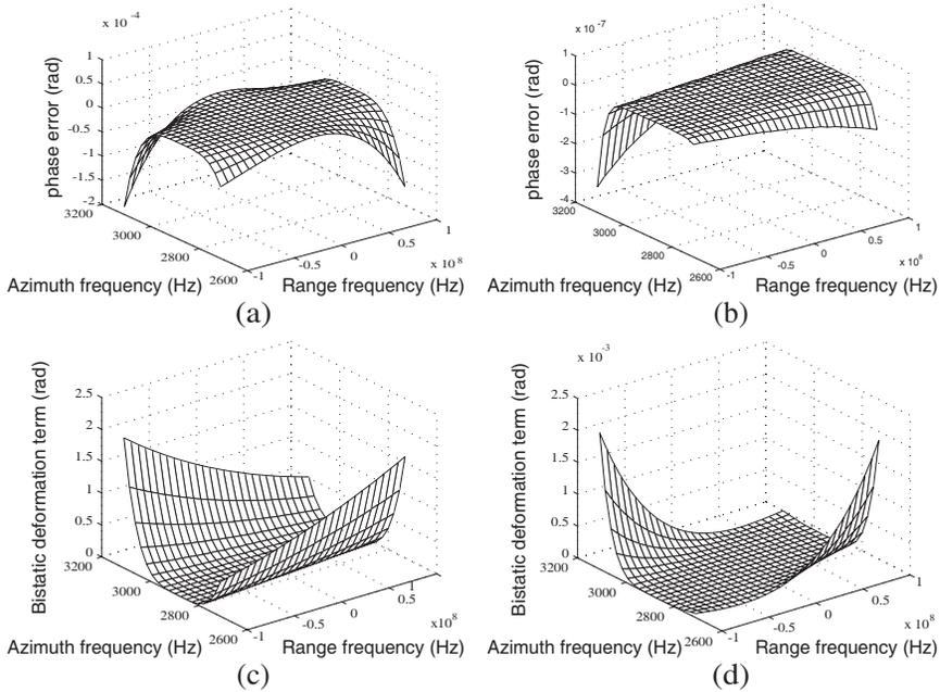
**Figure 4.** The phase error and BD phase term of AILBF using 1st-order and 2nd-order expansion of the Doppler frequency. (a) Phase error of 1st-order expansion; (b) Phase error of 2nd-order expansion; (c) BD term of 1st-order expansion; (d) BD term of 2nd-order expansion.
