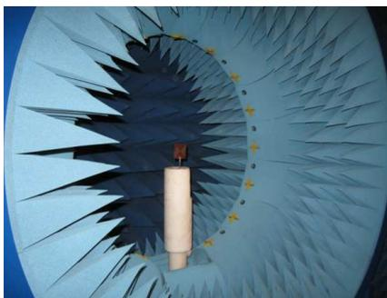
**Figure 6.** Antennas were tested through SATIMO anechoic chamber.
