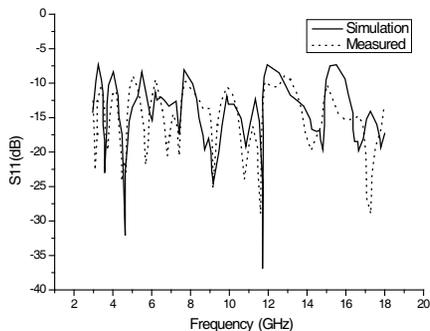
**Figure 7.** The return losses of the slot antenna without cavity.
