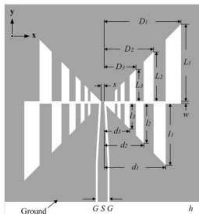
**Figure 2.** The dimension of the proposed antenna.
