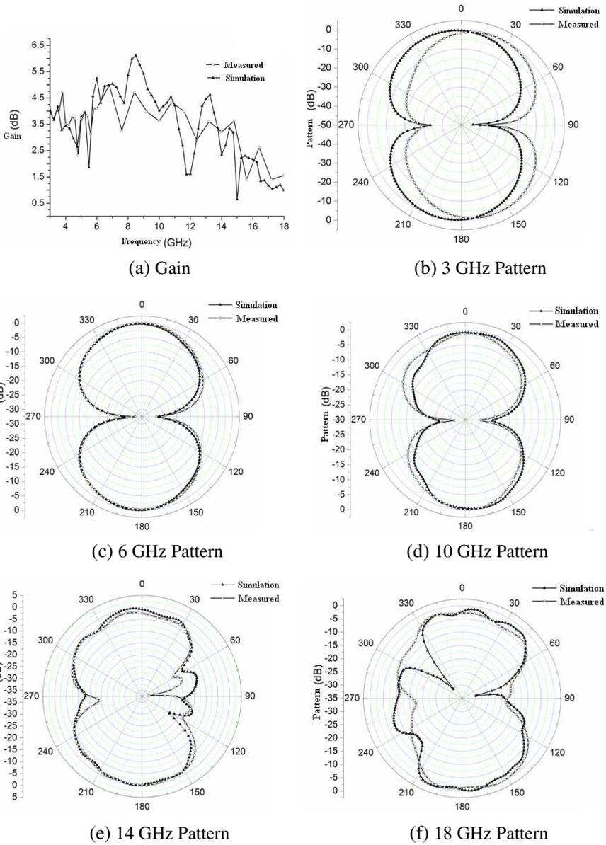
**Figure 8.** The radiation characteristics of the slot antenna without cavity.
