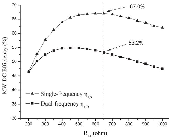
**Figure 4.** Measured MW-DC efficiency of the conventional rectifier with single- and dual-frequency microwave input at 17 dBm.
