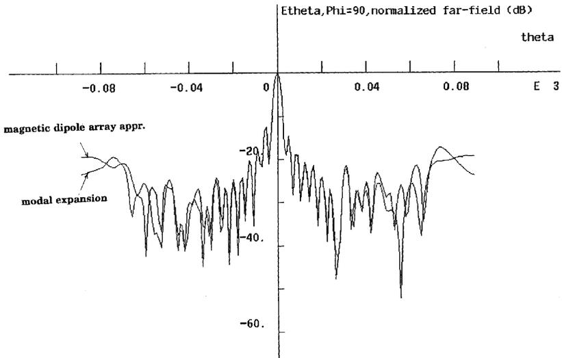
Figure 9. Co-polarization characteristic for  $\Phi = 90^\circ$  cut for a  $32 \times 32$  patch microstrip array using planar modal expansion method ( $81 \times 81$  data points) and equivalent magnetic dipole array approximation ( $41 \times 41$  data points).
