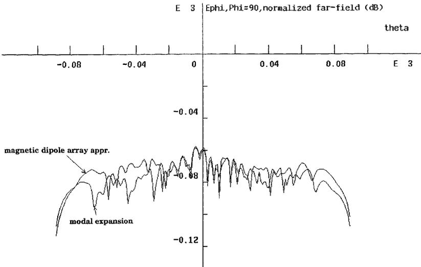
**Figure 11. Cross-polarization characteristic for  $\Phi = 90^\circ$  cut for a  $32 \times 32$  patch microstrip array using planar modal expansion method ( $81 \times 81$  data points) and equivalent magnetic dipole array approximation ( $41 \times 41$  data points).**
