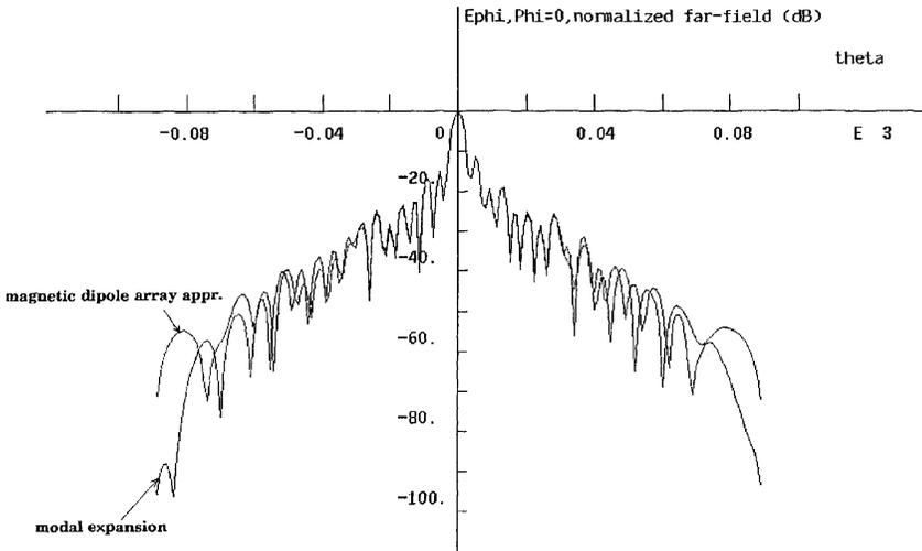
Figure 8. Co-polarization characteristic for  $\Phi = 0^\circ$  cut for a  $32 \times 32$  patch microstrip array using planar modal expansion method ( $81 \times 81$  data points) and equivalent magnetic dipole array approximation ( $41 \times 41$  data points)
