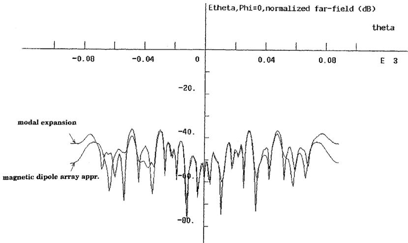
Figure 10. Cross-polarization characteristic for  $\Phi = 0^\circ$  cut for a  $32 \times 32$  patch microstrip array using planar modal expansion method ( $81 \times 81$  data points) and equivalent magnetic dipole array approximation ( $41 \times 41$  data points).
