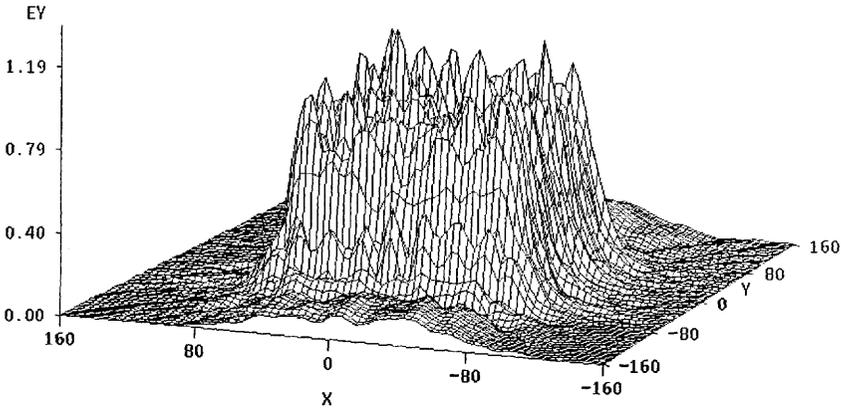
Figure 6. Amplitude of  $y$  component of measured electric near-field for a  $32 \times 32$  patch microstrip array.
