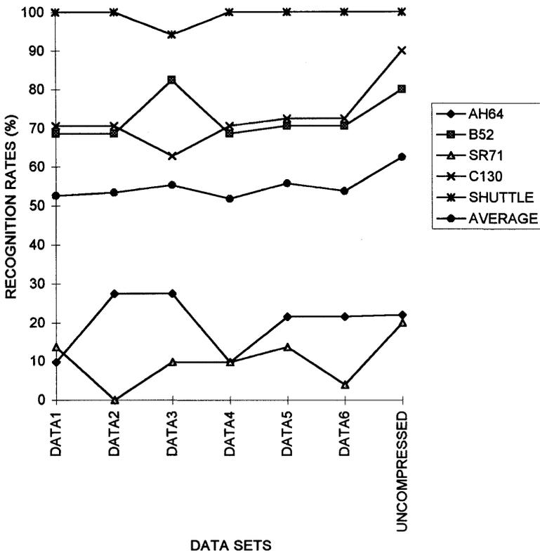
Figure 6. Recognition rates of several targets using different data sets. The unknown feature vectors are measured at  $\theta = 0^\circ, 20^\circ$ , while those stored in the data base are measured at  $\theta = 10^\circ$ .
