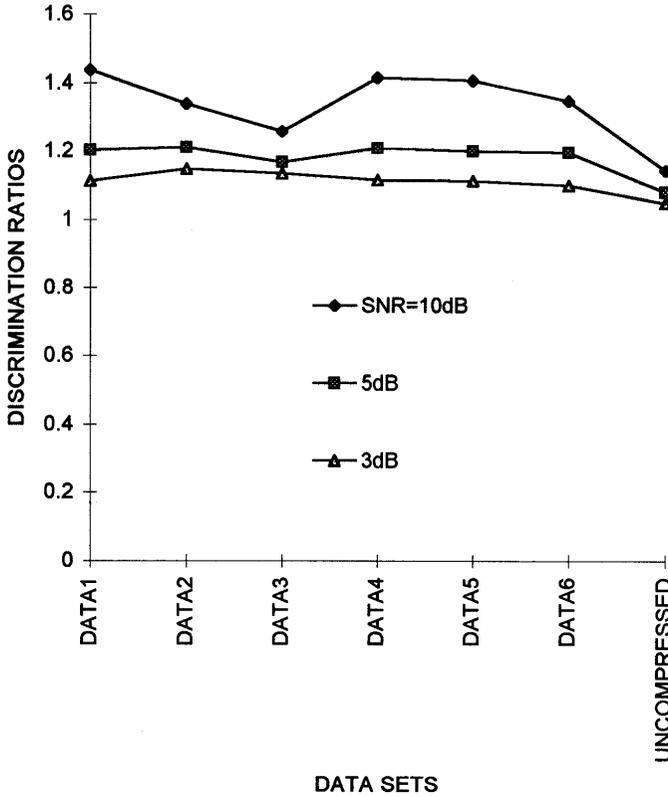
Figure 5. Averaged discrimination ratios using different data sets with several signal to noise ratios.
