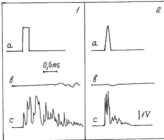
Figure 7. Effect of rectangular (1) and trapezoidal (2) pulses.  $B_o = 6.5$  T,  $J_M = 9$  A,  $f = 1211$  MHz; (a) current pulse, (b) RF envelope, (c) envelope of coil signal
