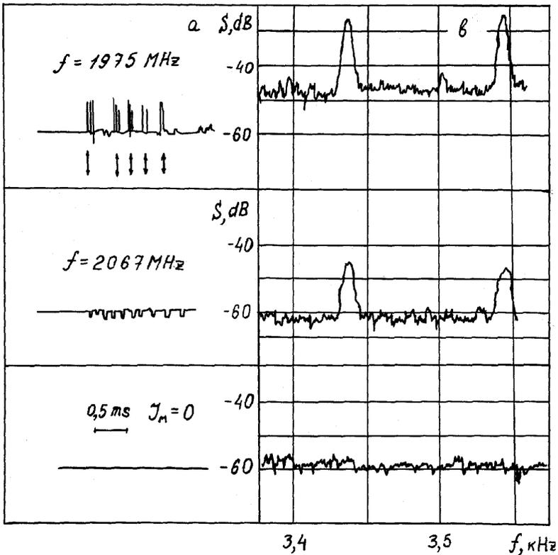
Figure 4. Signal envelope (a) and spectrum (b).  $B_0 = 6.5 \text{ T}$ ,  $J_M = 16 \text{ A}$ ,  $\tau_j = 120 \mu\text{s}$ .
