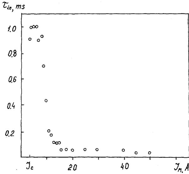
Figure 5. Instability development time vs. current strength.  $B_o = 4.5$  T,  $f = 1750$  MHz,  $\tau_j = 100\mu s$ .
