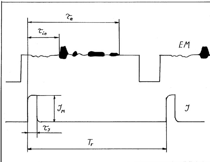
Figure 2. Schematic diagram of the wave envelope EM and current pulses  $j$  supported by temporal scales.
