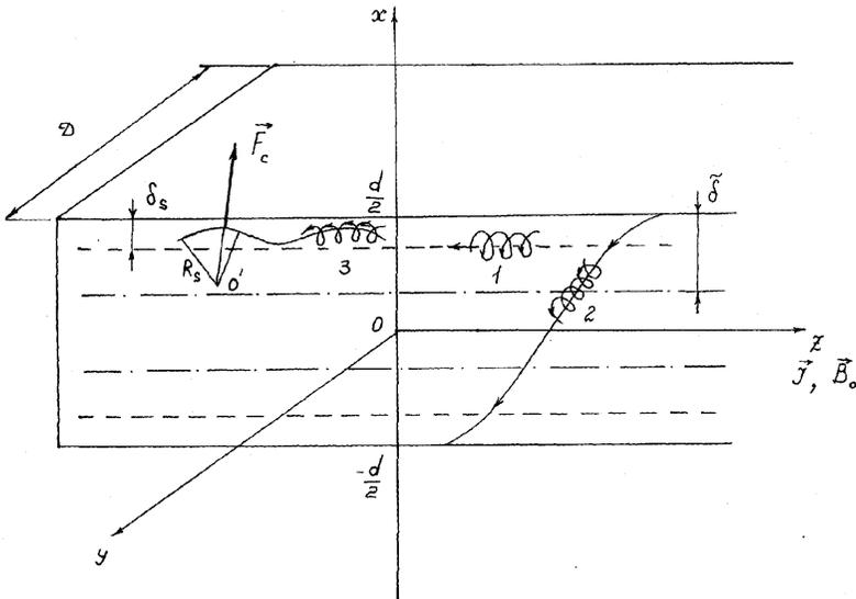
Figure 9. Movement of electrons in the metal plate. 1 - bulk electrons, 2 - flying electrons, 3 - trapped electrons.
