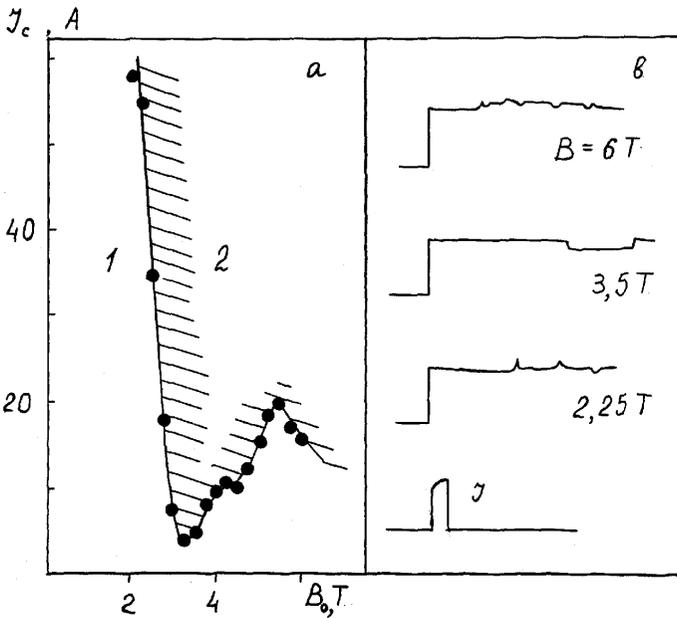
Figure 8. Critical current vs. magnetic induction (a) and the RF signal envelope at different  $B_o$ . (b)  $f = 1750$  MHz,  $\tau_j = 100 \mu s$ .
