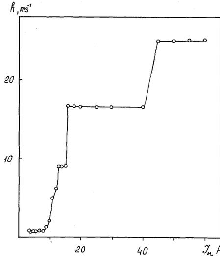
Figure 10. Kolmogorov entropy vs. current strength.  $B_o = 4.5T$ ,  $f = 1750$  MHz,  $\tau_j = 100\mu s$ .
