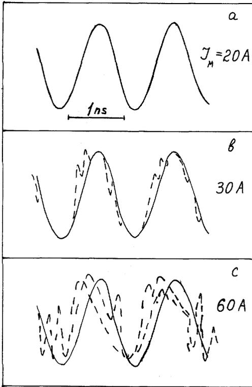
Figure 3. Unstable phase shift of RF signal.  $B_o = 7$  T,  $f = 794$  MHz,  $\tau_j = 160\mu\text{s}$ ;  $J_M = 20$  A (a), 30 A (b), 60 A (c).
