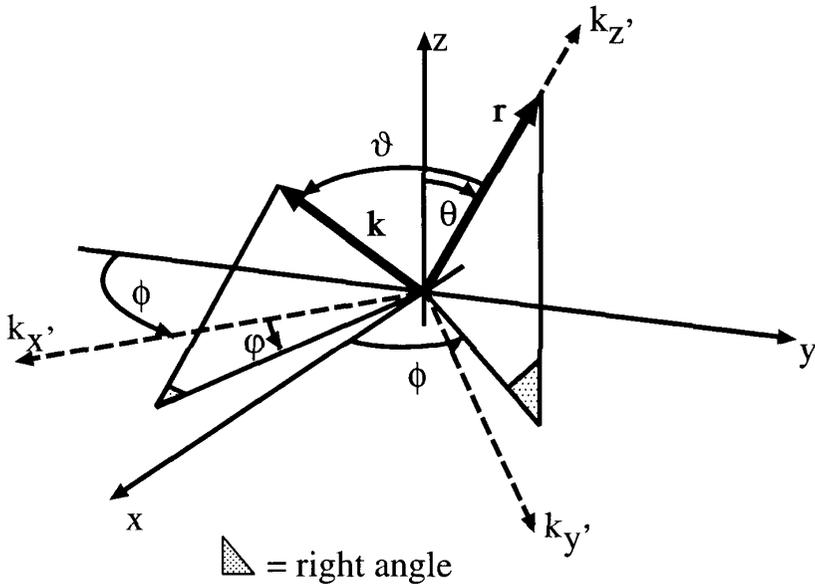
Figure 1. The rotated co-ordinate system (rotated axes are given as dashed lines). The  $x'$  axis lies in the  $x, y$  plane; the angles  $\varphi, \vartheta$  are spherical angles in the rotated system.
