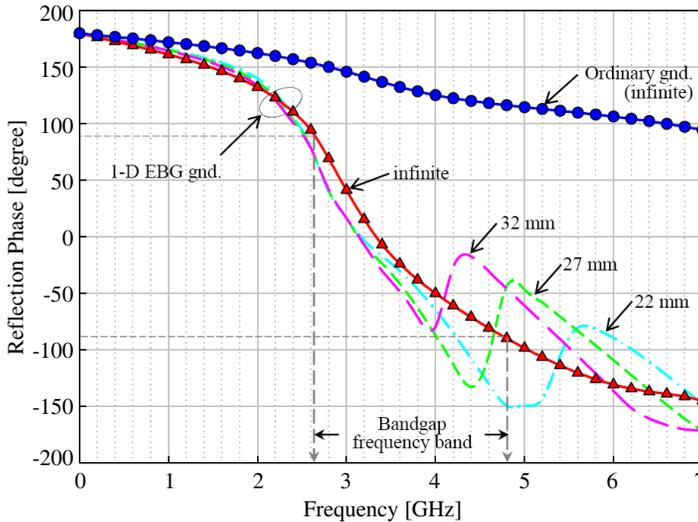
**Figure 4.** Reflection phases of the ground planes with and without the 1-D EBG structure obtained by the simulation method as shown in Figure 3(a). The reflection phases of the 22-, 27-, 32-mm-long and infinitely-long 1-D EBG ground planes are also compared to examine the effect of the ground length on the reflection characteristics.
