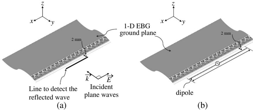
**Figure 3.** Configuration of the simulated structure and the simulation condition: (a) to obtain the reflection phase, (b) to find the input-match frequency band. ( $\vec{k}$ : wave vector,  $\vec{E}$ : electric field).
