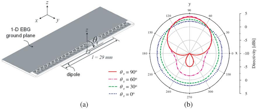
**Figure 6.** Radiation pattern of the dipole antenna with respect to the angle between the 1-D EBG ground plane and the dipole arms: (a) configuration of the ideal dipole antenna with 1-D EBG ground plane for the simulation study, (b) simulated radiation pattern on the  $xy$ -plane.
