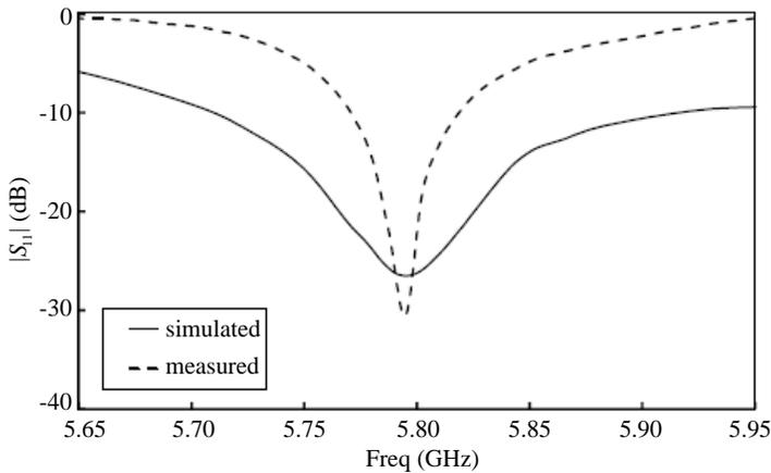
**Figure 9.** Reflection coefficient of six-sector antenna in operating mode.
