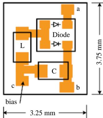
**Figure 2.** Structure of the proposed switching circuit.
