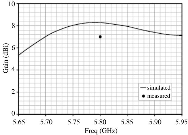
**Figure 13.** Gain of six-sector antenna in operating mode.
