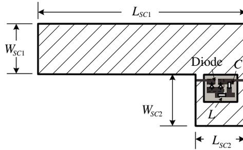
**Figure 3.** L-shaped coupling slot with switching circuit.
