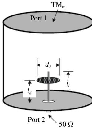
Figure 4. Disc-loaded probe.
