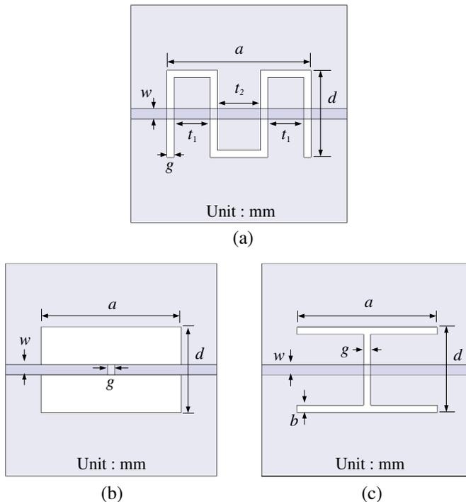
**Figure 1.** Three slotted-ground-plane resonators, where  $a = 20$ ,  $d = 12$ ,  $w = 1.5$ ,  $g = 1$ ,  $b = 1$ ,  $t_1 = 5$ ,  $t_2 = 6$ . (a) Proposed meandered slotted-ground-plane resonator. (b) Dumbbell-shaped resonators. (c) H-shaped resonators.
