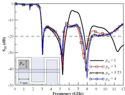
**Figure 10.** Dependence of the resonance frequency on the width ( $p_w$ ) of the aperture with  $p_l = 4.75$  mm.
