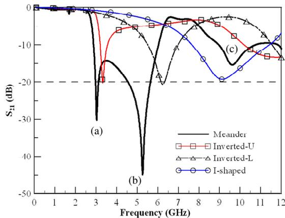
**Figure 4.** Simulated  $S_{21}$ -parameters of the slotted-ground-plane resonators, including the meandered, inverted-U, inverted-L and I resonators.
