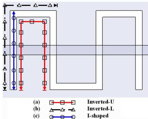
**Figure 3.** Three resonant paths of the meandered-slot resonator.
