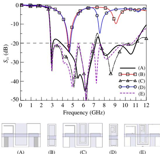
**Figure 14.** Simulated  $S_{21}$  of the five resonators, including the modified meandered slot (A), the C-like slot (B), the meandered slot with the C-like slot (C), the C-like slot with the spur slit (D), and the meandered slot with the spurred C-like slot (E).
