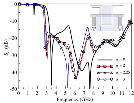
**Figure 13.** Simulated frequency response of the modified meandered slot with two rectangular-head slots whose dimension is  $a \times 5.25$  mm<sup>2</sup>.
