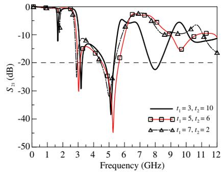
**Figure 7.** Simulated transfer characteristics of the test circuit by varying  $t_1$  when the slot width ( $g$ ) is fixed by 1 mm.
