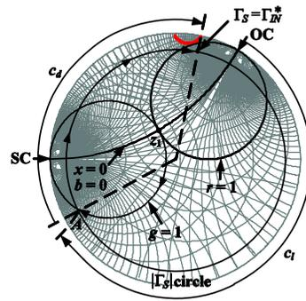
**Figure 9.** Meta-Smith chart solution using reciprocal CCITL open-circuited single-stub shunt tuners for the IMN at  $\phi = 30^\circ$ .
