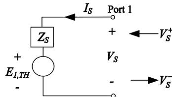
**Figure 4.** A Thévenin's equivalent circuit at the input port.
