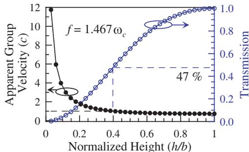
**Figure 4.** Group velocity and final transmission rate ( $|F_T|^2$ ) versus normalized height. Solid dots and open circles represent the group velocity ( $v_g = L/\tau_g$ ) and transmission, respectively.
