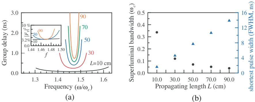
**Figure 5.** (a) Group delay versus frequency for five selected lengths. The inset in (a) shows the minimum transmission of 3.2% under off-resonant condition ( $1.467\omega_c$ ). (b) Superluminal bandwidth (black solid dots) and the shortest pulse width allowed for distortionless-superluminal propagation (blue solid triangles) versus propagating length. The pulse width is obtained based on the FWHM of a Gaussian profile.
