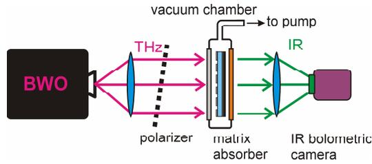
**Figure 4.** Optical scheme for imaging experiments. BWO — backward wave oscillator, vacuum chamber is supplied with input THz window (high density polyethylene) and with output IR window (coated ZnSe).
