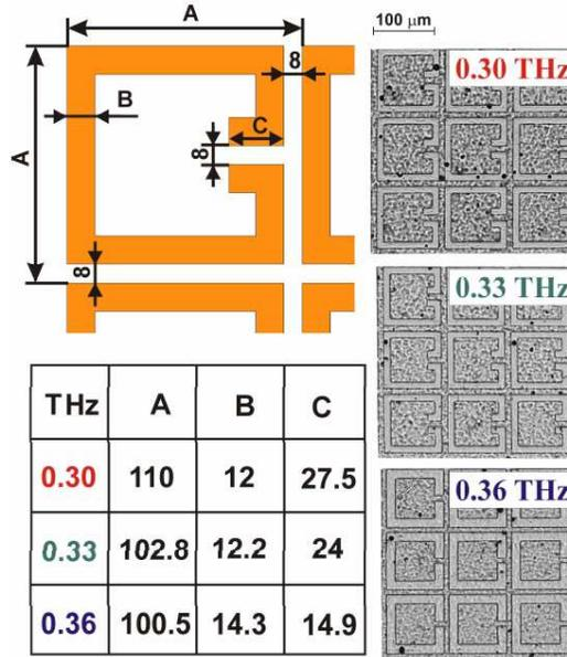
**Figure 2.** (left) Scheme and geometric parameters (in micrometers) of split-ring resonators optimized for absorption at 0.30, 0.33, 0.36 THz. (right) Photomicrographs of the topological pattern of fabricated splitting-ring resonators.
