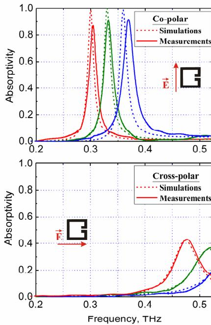
**Figure 3.** Absorptivity spectra of the absorbers for two orthogonal polarizations. Simulated and measured spectra are shown by dashed and solid lines respectively. Polarization directions relative to SRR gap for co-polar ( $\mathbf{E} \perp$  SRR gaps) and cross-polar ( $\mathbf{E} \parallel$  SRR gaps) polarization modes are shown in insets.
