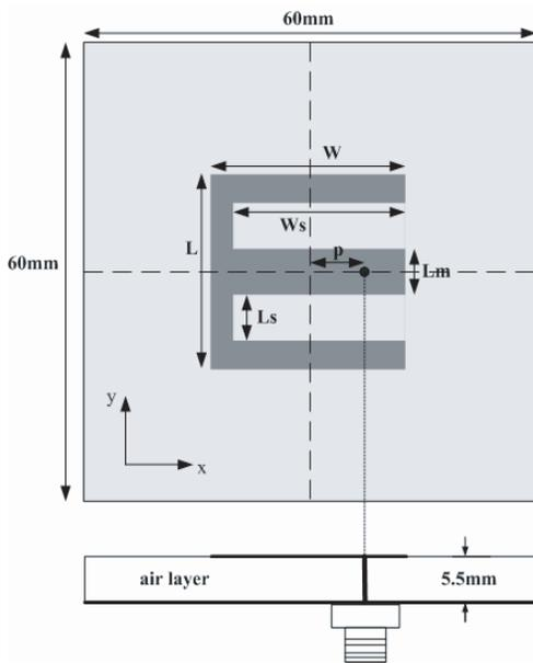
**Figure 5.** Geometry of the E-shaped patch antenna.
