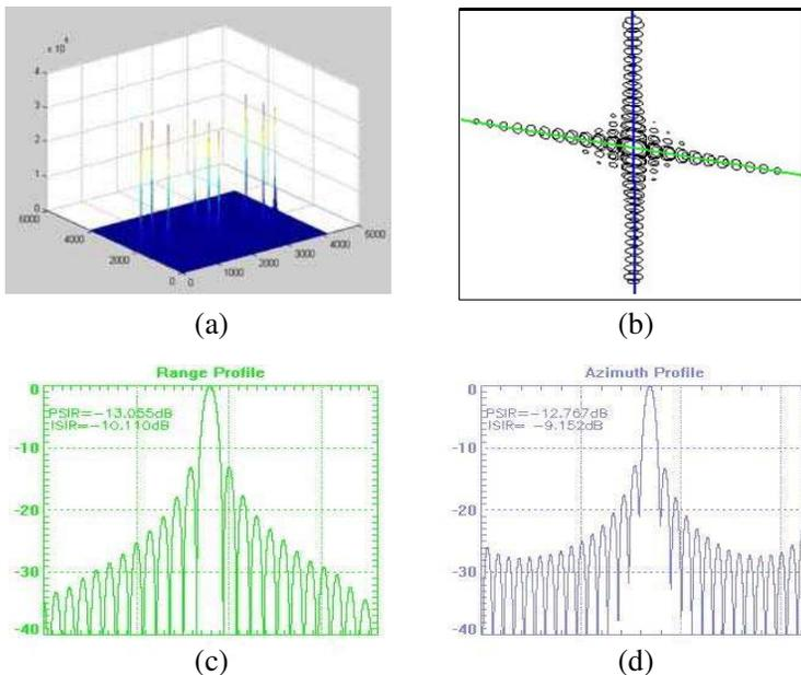
**Figure 8.** Imaging results and image quality inspection for ellipse trajectory mode.
