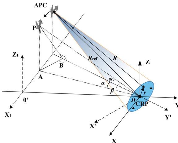
Figure 1. Spotlight mode SAR geometry.
