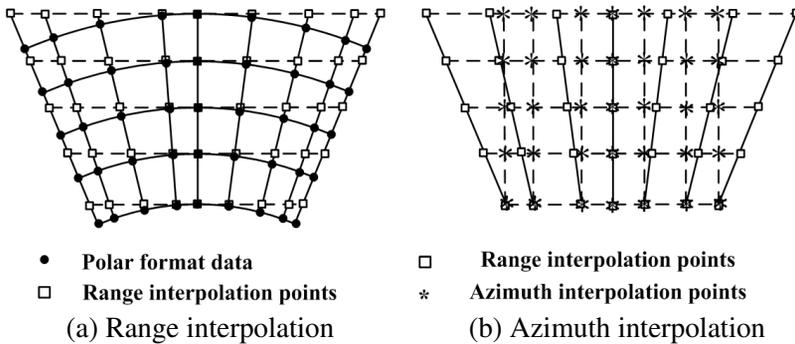
**Figure 2.** Interpolation from polar format to rectangular format.
