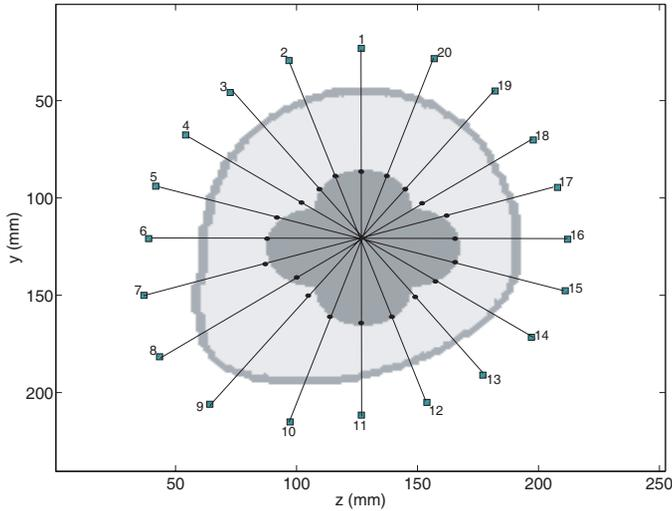
**Figure 6.** Contour samples (dots) evaluated for contour  $\Gamma_{23}$  of model 3 when the algorithm uses a single reference signal constructed from the reflection off of a dielectric slab with  $\epsilon_r = 37.4$ ,  $\sigma = 4.2 \text{ S/m}$ .
