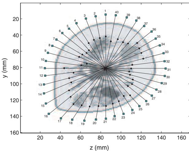
**Figure 9.** Contour samples (dots) evaluated for contour  $\Gamma_{23}$  of model 5 when the algorithm uses a two different reference signals constructed from the reflections off of a dielectric 3 mm slab with  $\epsilon_r = 37.5$ ,  $\sigma = 4.2\text{S/m}$ . Only one set of reference signals is acquired when a 3 mm homogeneous dielectric slab is illuminated with the 4.62 GHz BW.
