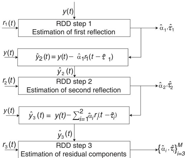
**Figure 2.** Flow-chart of the three-step procedure used to estimate the scaling factor  $\alpha$  and *TOA* parameter  $\tau$  for each reflection contained in the backscattered data  $y(t)$  recorded by a sensor. At each step, *a priori* information about a region (e.g., geometrical and/or dielectric properties) may be incorporated into the reference signal  $r_i(t)$  used by the reflection data decomposition algorithm.
