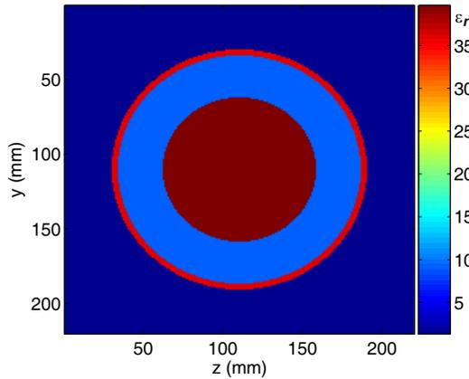
**Figure 3.** Relative permittivity profile of model 1. The skin layer is 2 mm thick with  $\epsilon_{r1} = 36.0$ ,  $\sigma_1 = 4.0$  S/m; the middle layer is 14 mm thick with  $\epsilon_{r2} = 9.0$ ,  $\sigma_2 = 0.4$  S/m; and the center layer is 24 mm thick with  $\epsilon_{r3} = 40.0$ ,  $\sigma_3 = 3.2$  S/m.
