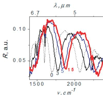
**Figure 8.** Smooth tuning of the resonance peak from  $1700$  to  $1880 \text{ cm}^{-1}$  in the experimental reflection spectra of the FP resonator (from Fig. 5) with a maximal relative shift of  $\Delta\lambda/\lambda = 10\%$ .
