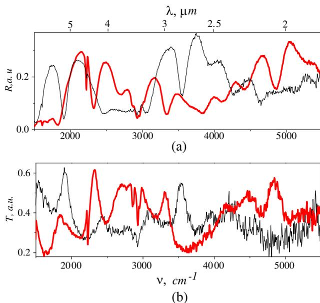
**Figure 4.** FTIR (a) Reflection and (b) Transmission spectra of the FP resonator with LC filler for  $E$  (thick line) and  $H$  (thin line) polarizations in the absence of an applied electric field. The resonator parameters are: width of Si walls,  $d_{Si} = 1 \mu\text{m}$ , cavity width,  $d_{cav} = 4 \mu\text{m}$ .
