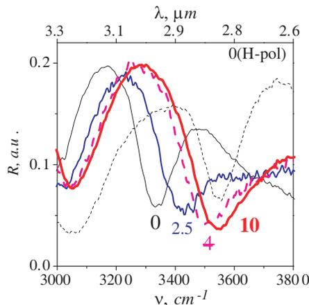
**Figure 6.** Smooth tuning of the position of the resonance peak from  $3330\text{ cm}^{-1}$  to  $3550\text{ cm}^{-1}$  for  $E$ - and  $H$ -polarization (dotted line). The applied voltage is shown in volts beside each curve.
