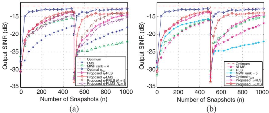
**Figure 6.** Output SINR performances evaluation of the proposed adaptive combination approach with iterative algorithms in a nonstationary scenario. (a) Relationship of the combined filters and their component filters. (b) Comparison of the proposed iterative algorithms with other adaptive algorithms.
