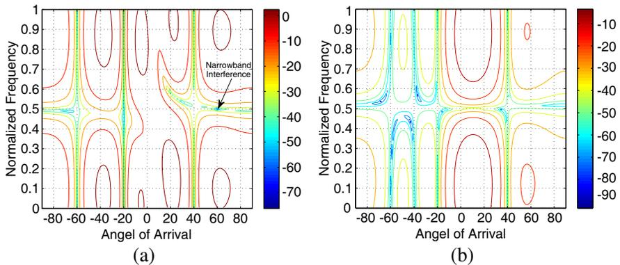
**Figure 3.** Two-dimensional beam pattern of the proposed beamformer. (a) There are 3 wideband interferences and 1 narrowband interference. (b) There are 4 wideband interferences, one of them comes from  $-40^\circ$  with SIR = -40 dB and 1 narrowband interference which is the same as in Figure 3(a).
