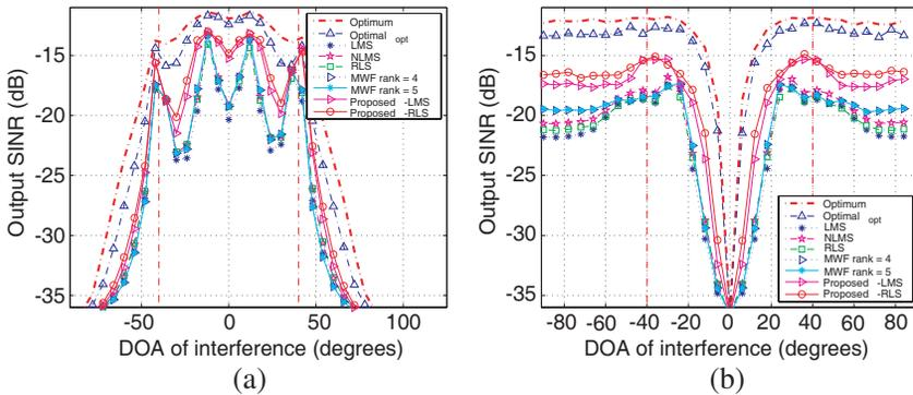
**Figure 7.** DOAs of the interference versus output SINRs, when the DOA of desired signal arrives from two directions (a) The DOA of desired signal is  $\theta_d = 90^\circ$ . (b) The DOA of desired signal is  $\theta_d = 0^\circ$ .
