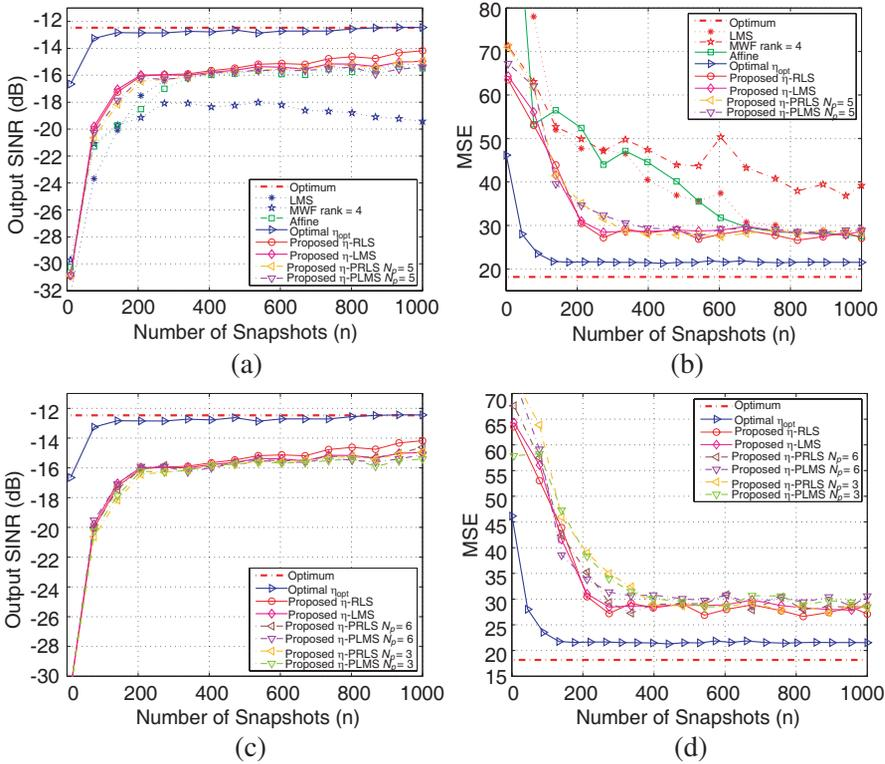
**Figure 5.** Output performances evaluation of the proposed adaptive combination approach with iterative algorithms in a mixed bandwidth interference environment. (a) Relationship of the combined filters and their component filters. (b) MSE of the filters in the left figure. (c) Comparison of the proposed iterative algorithms with their partially updated  $\hat{\eta}(n)$  algorithms. (d) MSE of the filters in the left figure.
