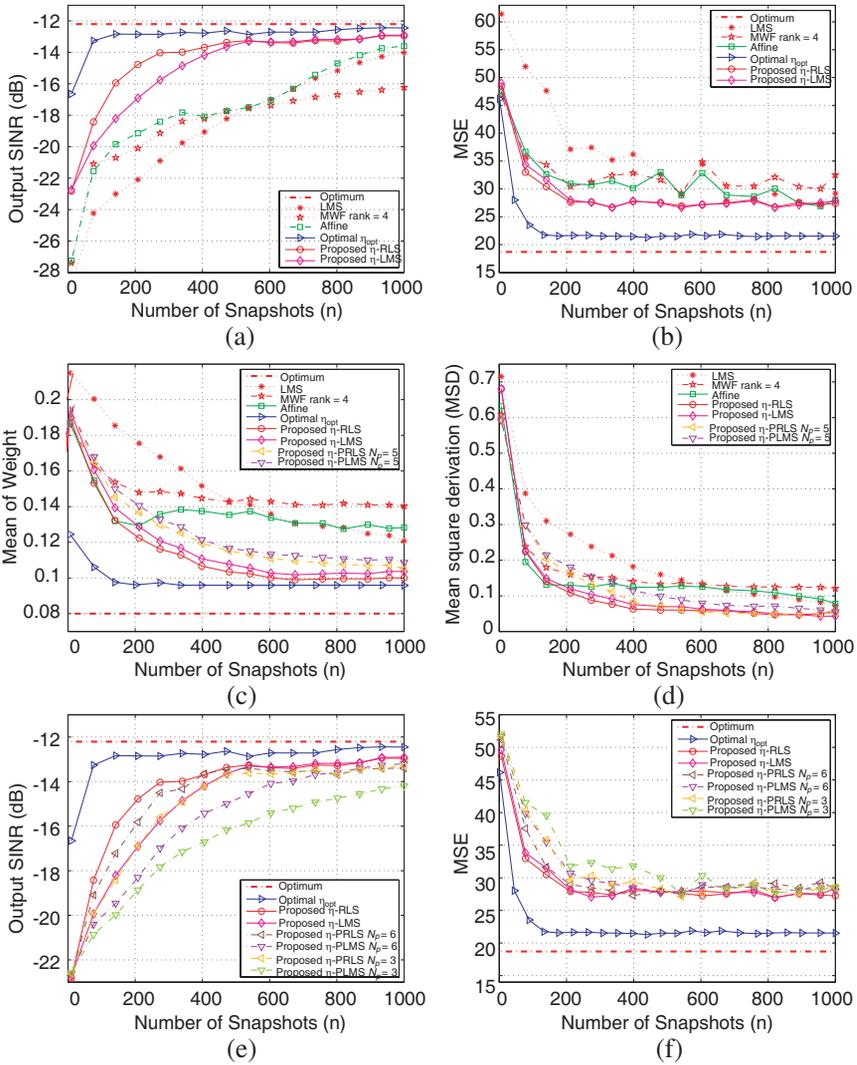
**Figure 4.** Output performances evaluation of the proposed adaptive combination approach with iterative algorithms in stationary environment. (a) Relationship of the combined filters and their component filters. (b) MSE of the filters in the left figure. (c) Mean value of the 1st entry of weight. (d) Mean square derivation of the filters. (e) Comparison of the proposed iterative algorithms with their partially updated  $\eta(n)$  algorithms. (f) MSE of the filters in the left figure.
