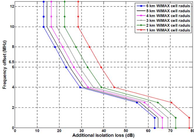
**Figure 10.** The required additional isolation loss versus the frequency offset (WiMAX is 5 MHz).
