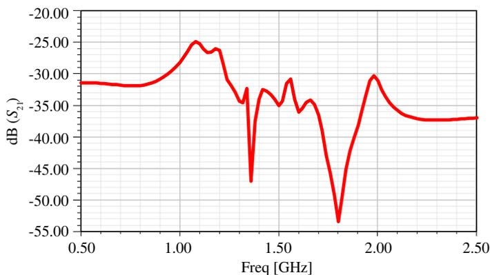
**Figure 11.** Isolation between ports versus frequency.
