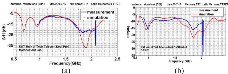
**Figure 2.** Return loss as a function of frequency. (a) Port 1. (b) Port 2.  $L_D = 115$  mm,  $W_D = 190$  mm,  $L_{n1} = 20$  mm,  $W_{n1} = 110$  mm,  $L_{n2} = 15$  mm,  $W_{n2} = 45$  mm,  $L_s = 10$  mm,  $W_s = 8$  mm,  $L_g = 290$  mm,  $W_g = 220$  mm,  $L_{ap} = 100$  mm,  $W_{ap} = 10$  mm,  $L_1 = 45$  mm,  $L_2 = 40$  mm,  $W_1 = 3.06$  mm,  $W_2 = 0.7$  mm,  $L_{S1} = 75$  mm,  $L_{S2} = 115$  mm,  $L_h = 30.24$  mm,  $L = 5$  mm,  $h = 17$  mm.
