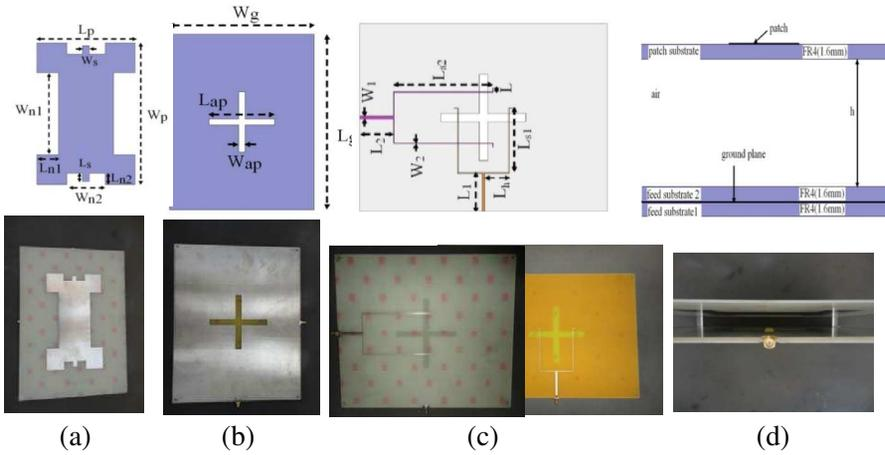
**Figure 1.** Geometry of the proposed antenna element. (a) Patch in layer 1. (b) Coupling slots in ground plane. (c) Microstrip-line feed network. (d) Side view of the antenna.
