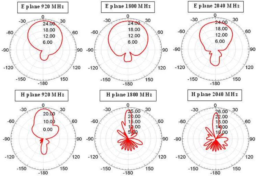
**Figure 12.** Simulated radiation patterns in  $E$  and  $H$  planes of the antenna at 920 MHz, 1800 MHz, and 2040 MHz.
