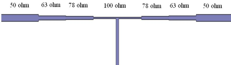
**Figure 6.** Three section Chebyshev transformer for impedance matching.
