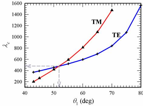
**Figure 5.** The calculated critical wavelength as a function of the angle of incidence for the 50/50 beam splitting. Both  $TE$  and  $TM$  curves have an crossover at  $\theta_1 = 51.8^\circ$  and  $\lambda_c = 478$  nm.
