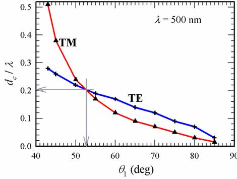
**Figure 3.** The calculated critical thickness as a function of the angle of incidence for the 50/50 beam splitting. Both  $TE$  and  $TM$  curves have an intersection at  $\theta_1 = 52.6^\circ$ , and  $d_c/\lambda = 0.21$ .
