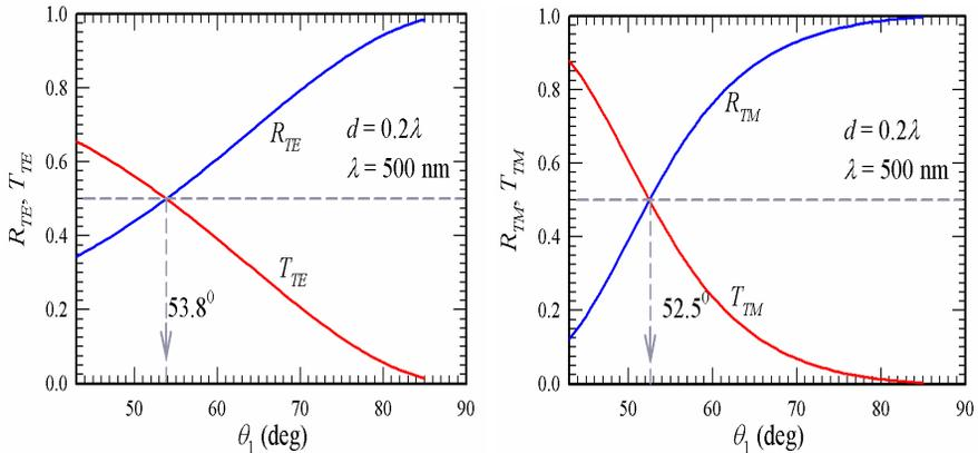
**Figure 6.** The calculated angle-dependent reflectance and transmittance for the  $TE$  wave and  $TM$  waves. The  $TE$ -wave critical angle is  $\theta_c = 53.8^\circ$  and  $TM$ -wave critical angle is  $\theta_c = 52.5^\circ$ .
