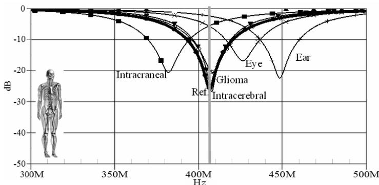
**Figure 4.** Simulated return losses for the implanted antenna inside the head of the male anatomical computer model. The gray vertical line corresponds to the MISC reference frequency. The thick black line corresponds to the response of the liquid simulating the head reference tissue.
