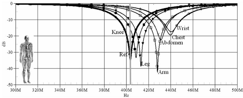
**Figure 5.** Simulated return losses for the implanted antenna located in several subcutaneous positions inside the male anatomical computer model (Figure 3). The gray vertical line corresponds to the MISC reference frequency. The thick black line corresponds to the response of the liquid simulating the body reference tissue.
