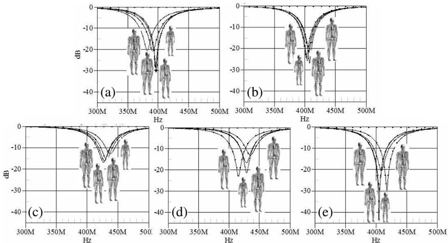
**Figure 7.** Simulated return losses for the antenna implanted inside the head for the four anatomical computer models. Results for (a) intracranial, (b) intracerebral, (c) ear, (d) eye and (e) glioma regions are presented.
