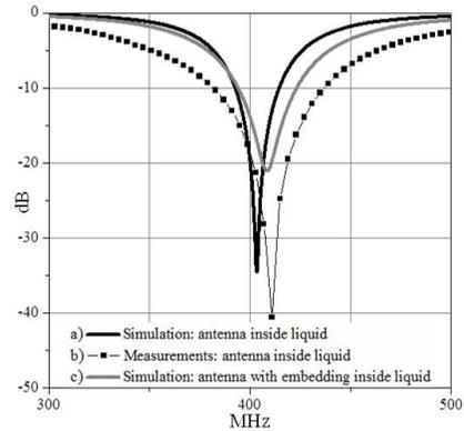
**Figure 2.** Simulated and measured return losses of the antenna design.
