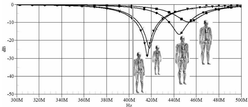
**Figure 10.** Simulated return losses for the antenna implanted inside the abdomen for the four anatomical computer models. The gray vertical line corresponds to the MISC reference frequency. The antenna was located 8 mm from the skin-air interface.
