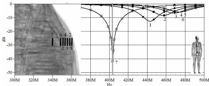
**Figure 8.** Simulated return losses for the antenna implanted inside the chest of the female anatomical computer model. The gray vertical line corresponds to the MISC reference frequency. The antenna was positioned 4 mm (1), 8 mm (2), 12 mm (3), 16 mm (4), 20 mm (5), 24 mm (6) and 40 mm (7) from the air-skin interface.
