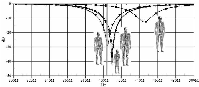
**Figure 9.** Simulated return losses for the antenna implanted inside the arm for the four anatomical computer models. The gray vertical line corresponds to the MISC reference frequency. The antenna was located 15 mm from the skin-air interface.
