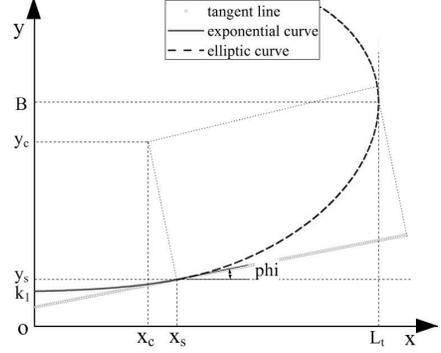
**Figure 2.** The structure geometry for the tapered line.
