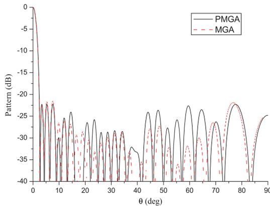
**Figure 5.** Best radiation patterns obtained by PMGA and MGA.
