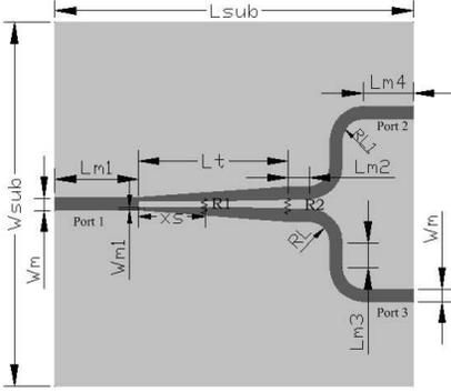
**Figure 1.** Geometry of the proposed power divider.
