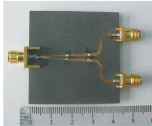
**Figure 7.** Photograph of the proposed power divider.
